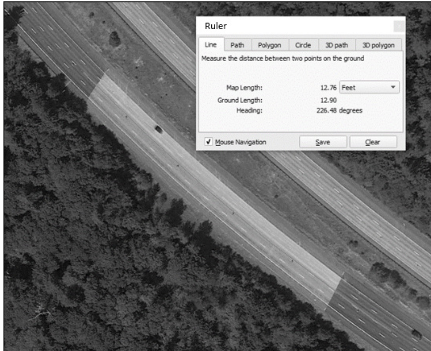
Figure 21. Screenshot. Example of freeway segment outside barrier offset measurement (Google 2023).
