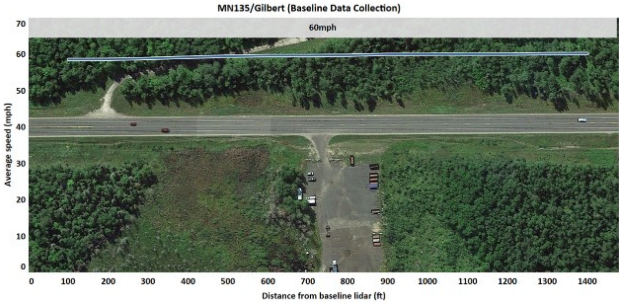
Figure 17 Average Speed Profile as Vehicles Transit through 60 mph Speed Zone on MN135/Gilbert Corridor
