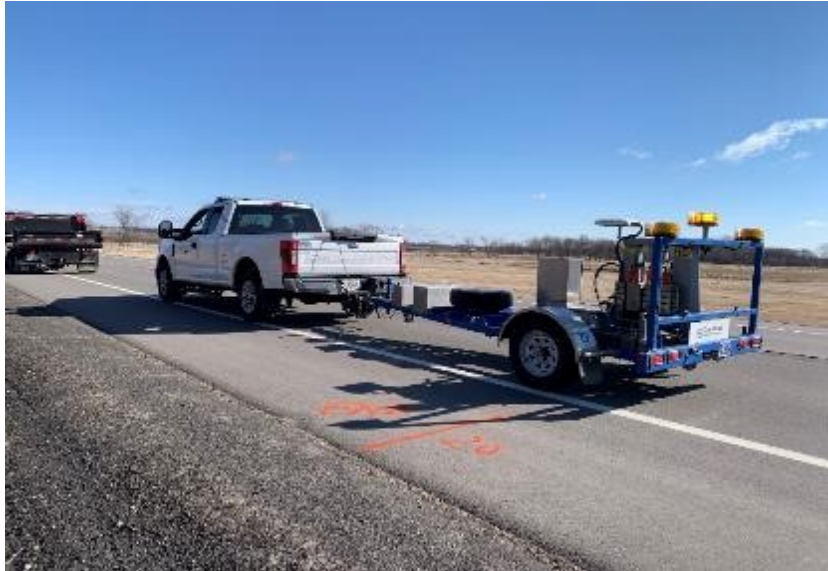
Figure 64. Dynatest model 8002 falling weight deflectometer device from MnDOT
