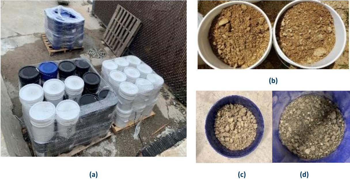
Figure 13. (a) Storing the collected material, (b) Class 5 limestone, (c) subgrade soil, and (d) FDR
