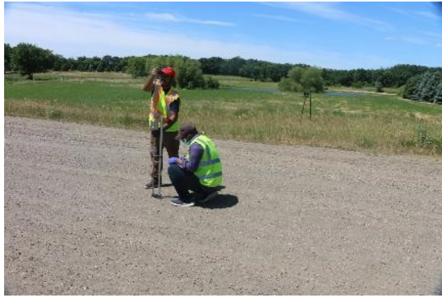
Figure 52. Conducting DCP test on Base One stabilized FDR base layer
