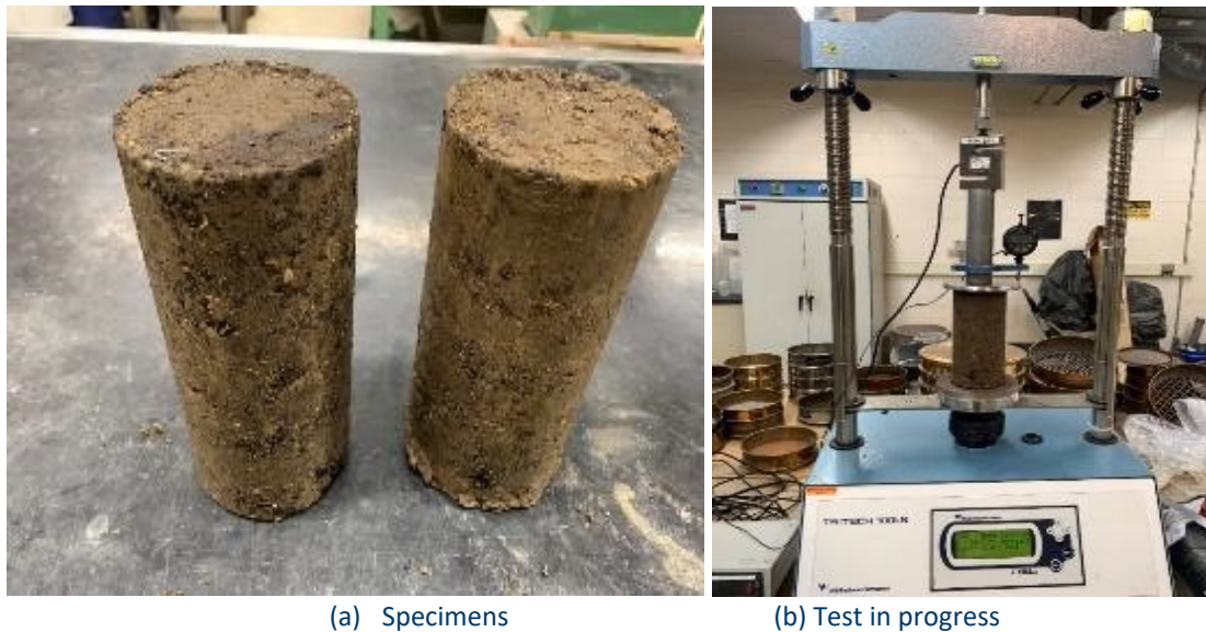
Figure 22. (a) Stabilized FDR-soil specimens (b) performing UCS test
