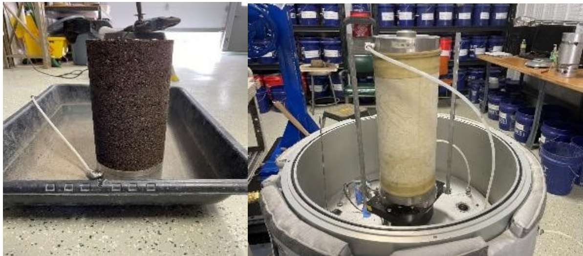
Figure 78. Sample preparation for repeated load triaxial test (a) compacted FDR aggregate specimen (b) placed on top of the bottom platen mounted to the lower pedestal of the triaxial chamber
