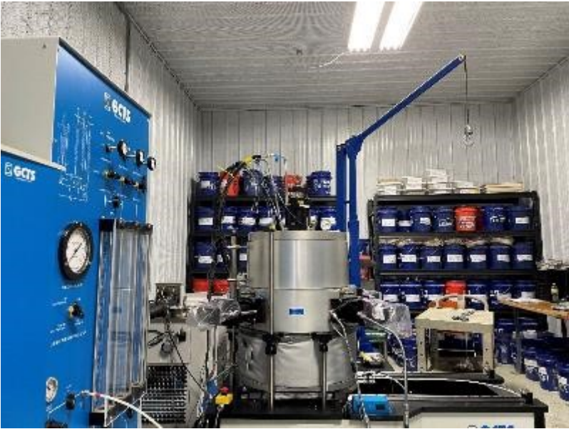
Figure 79. Repeated load triaxial test setup
