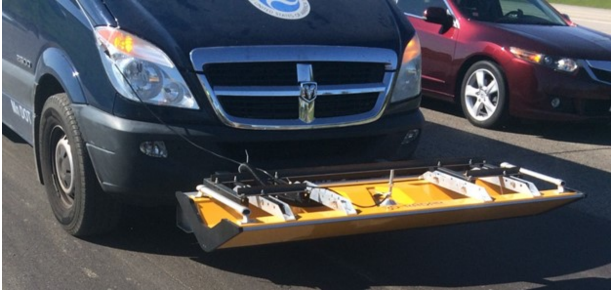
Figure 4.18 GPR Antenna (Yellow Object Mounted to the Front of the Van) During Data Collection on Asphalt Pavement Construction
