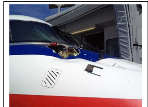
This Embraer 135 hit a common loon at 2900 feet on final approach into a Michigan airport in May 2014. The 12-lb bird penetrated the bulkhead and splattered blood on the flight crew. The aircraft landed safely. Aircraft was out of service over 6 months for repairs to radome, fuselage and instrument panels. Photo by aircraft owner.
