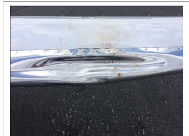
A Cessna 560 struck a turkey vulture at 1600 feet AGL on approach to a general aviation airport in Florida, July 2014. The leading edge of wing and deicing unit were damaged. Repair costs were $162,000 and aircraft was out of service for 2 months. Photo by aircraft owner.
