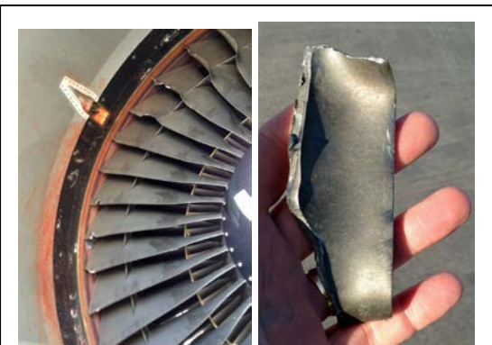
A Boeing 767 departing a western airport in June 2014 struck several Canada geese at 400 feet AGL. The #2 Engine exhibited severe vibrations and the pilot made an emergency landing. Parts of 2 Canada geese and 2 fan blades were recovered from runway. Wing flaps were also damaged. Repair costs were $3.9 million. Photo by airport Operations personnel.
