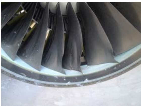
An Airbus 319 ingested a red-tailed hawk in the #1 engine during the take-off run from a southern U.S. airport, August 2014. The pilot aborted take-off at 143 knots. Aircraft was out of service 120 hours; cost of engine replacement and other repairs was $6.5 million. Red-tails are the hawk species most frequently struck by civil aircraft in USA (Table 17). Photo, aircraft operator.
