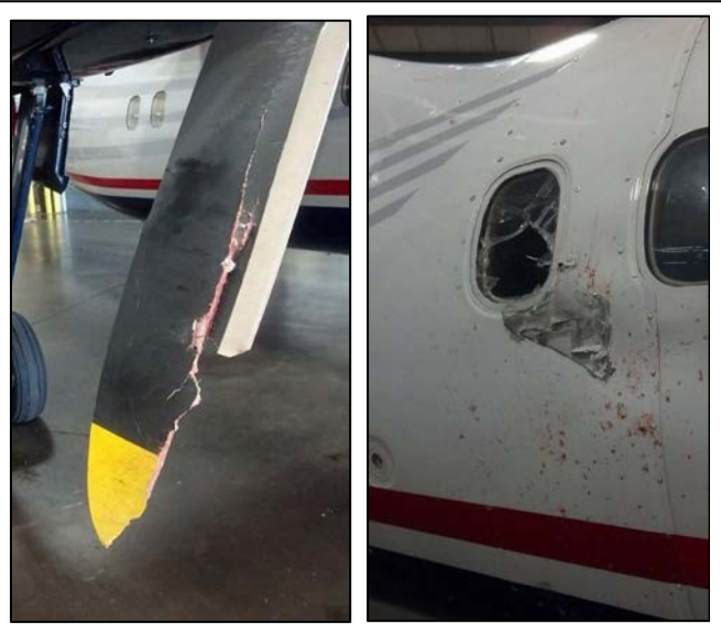
A DHC8 DASH aircraft struck several Canada geese during the initial take-off run from a Pennsylvania airport at dawn on 10 August 2014. The fuselage and a passenger window were damaged by a goose that was slung into side of aircraft after striking a propeller blade. The damaged propeller caused strong engine vibrations and pilot aborted take-off at 40 knots. Photo by aircraft owner.
