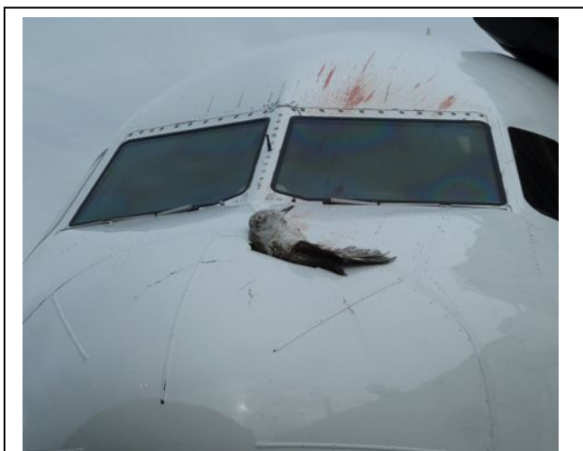
An Airbus 320 departing an east coast airport in March 2014 struck a sub-adult herring gull at 300 feet AGL. The bird became wedged in the radome and spattered blood over the left windshield. The pilot declared an emergency and diverted to a nearby major airport where a safe landing was made. The aircraft was out of service for 7 hours while the radome was replaced. Photo by Stan Nowak.
