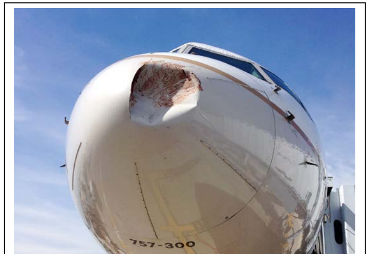
A Boeing 757 struck a bird at 4600 feet AGL during climb out from a western airport in September 2014. Flight crew detected no abnormalities and continued to destination airport where large dent in radome was revealed. Bird remains were recovered and identified as Franklin's gull by Smithsonian Feather Lab. Aircraft was out of service 24 hours and repair costs were $30,000. Photo, USDA.
