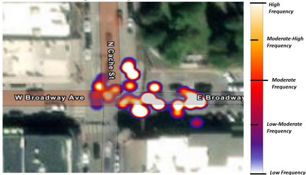
Figure 55 Heatmap of Conflicts
