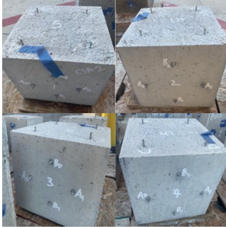
Figure 11.13: Completed concrete exposure block – CSA2
