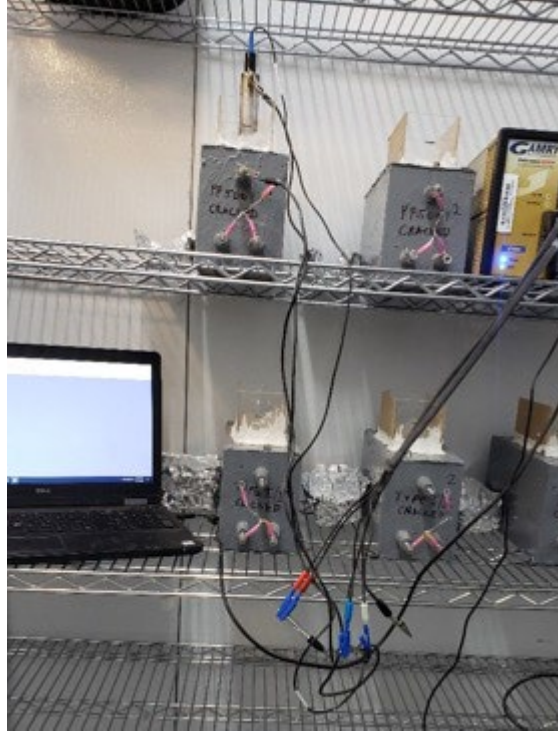
Figure 9.4: Configuration for microcell corrosion measurement
