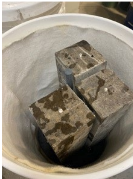
Figure 11.8: Container storing prisms for ASTM C1293
