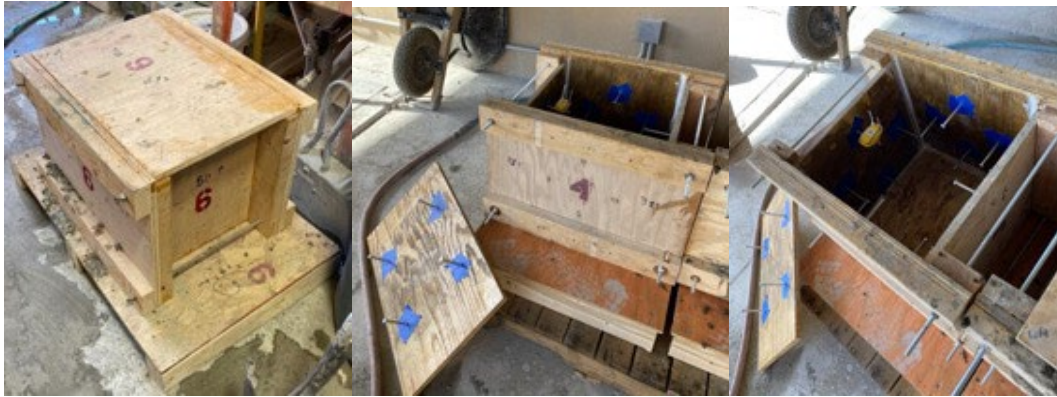
Figure 11.9: (1) Exterior View of 16 x 16 x 16 in Wooden Mold (2) Side View of Wooden Mold (3) Interior View of Wooden Mold.
