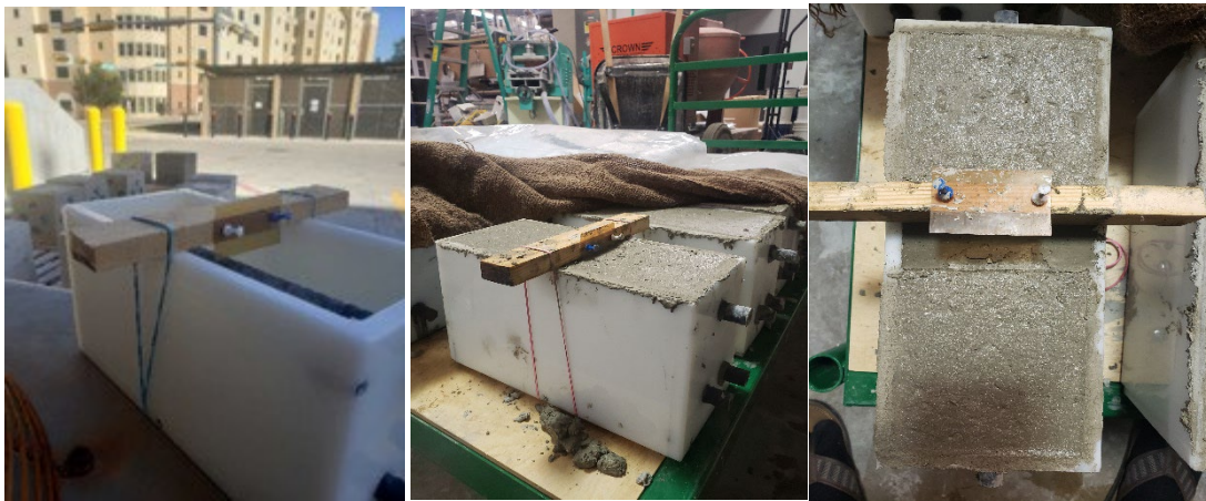
Figure 9.2: Set-up for crack introduction
