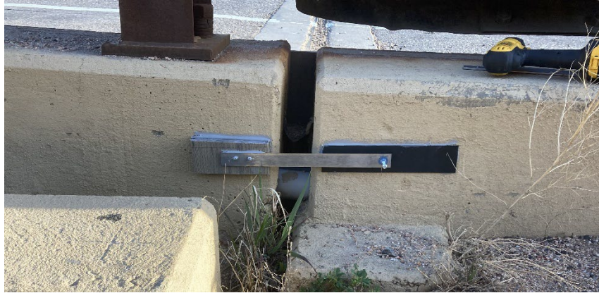
Figure 3-8 Scratch gauge installed on a bridge
