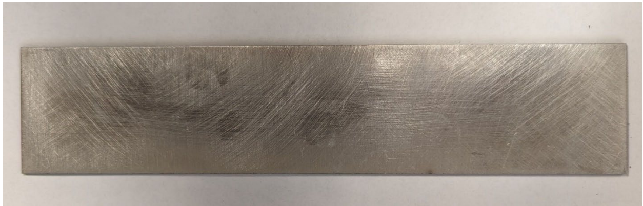
Figure B-1 A scratch gauge that has been scuffed by sandpaper
