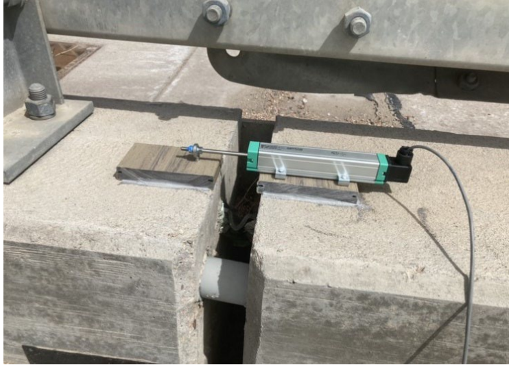
Figure 3-5 Installed potentiometer linear position sensor
