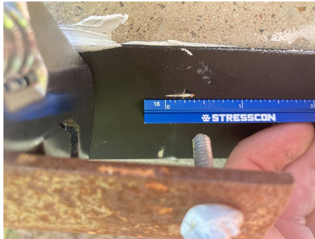
Figure 5-1 Scratch gauge measurement
