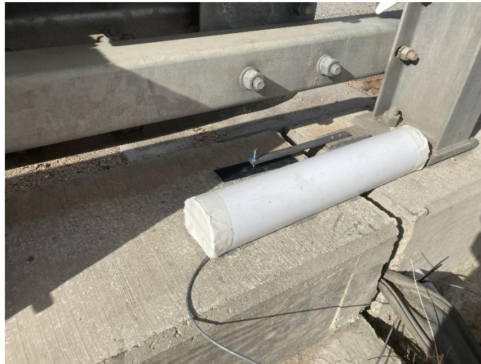
Figure 3-9 Equipped Potentiometer with weatherproofing installed
