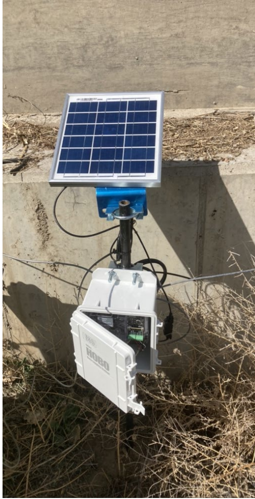
Figure 3-10 DAQ as installed on-site with solar panel
