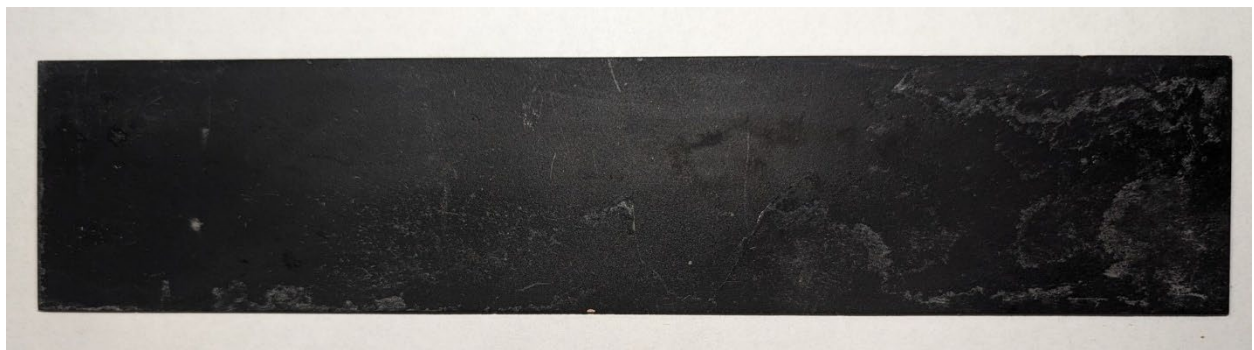
Figure B-2 A scratch gauge that has been spray painted with a black enamel coating
