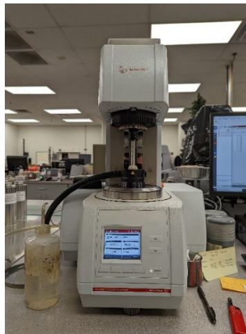
Figure 1 Anton Paar Smart Pave 102e rheometer used for DSR testing at CDOT's Bituminous Lab
