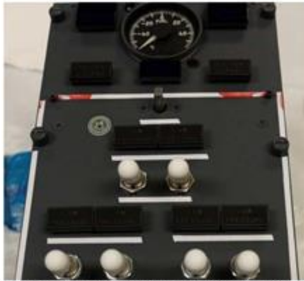
Figure 6: Indications of ingress observed on fuel control panel after set of 1 application
