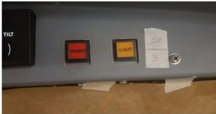
Figure 12 - Test 2 – results for 0 and 20 J/cm 2 - Warning and Caution pushbuttons
