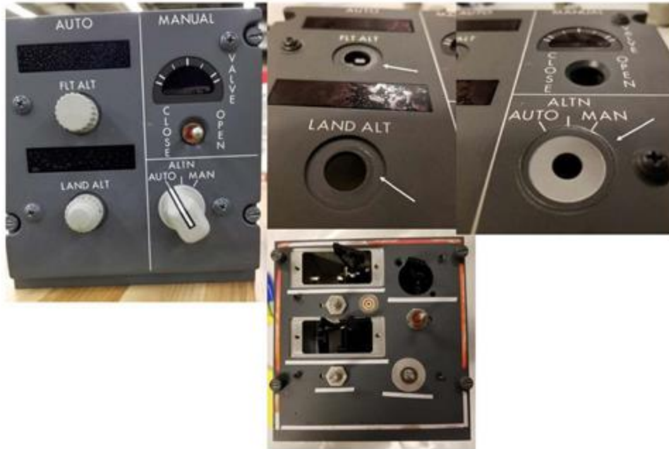
Figure 33. Left: Photo of [REDACTED] P5-6 Cabin Pressure Selector Panel after 130 applications of Calla 1452. Residue was visible on the display screens. Top Center and Right: Photos of the obverse side of the display plate after removal, showing residue on the display screens and wet residue or fluid under the knobs (white arrows). Bottom Center: Photo of the housing front plate with display plate removed. Indicator tape was red in many locations, indicating fluid ingress between the display plate and housing front plate. Evidence of moisture ingress behind the front plate was not observed visually, even with the aid of a flashlight. Due to the design of the housing, further non-destructive disassembly was not possible.
