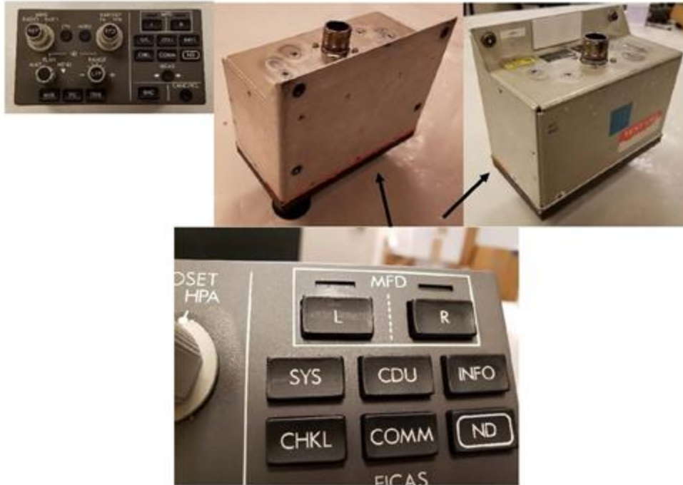
Figure 65. Photos showing condition of [REDACTED] DCP after 210 th application of Calla 1452. Top Row: External condition of the DCP. The red tape (black arrows) along the underside edges of the housing indicated fluid intrusion between the housing and mounting provisions. Bottom: Photo showing the light plate. Residue (white arrows) was present on much of the DCP surface, especially around knobs and buttons.
