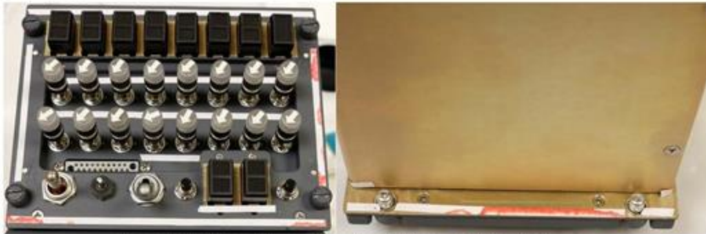
Figure 7: Indications of ingress observed on ACP after set of 4 applications
