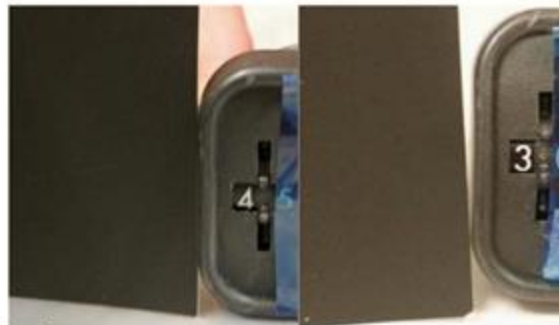
Figure 4: [redacted] black color scheme; initial (left), after 20 cycles of 70% IPA (right)
