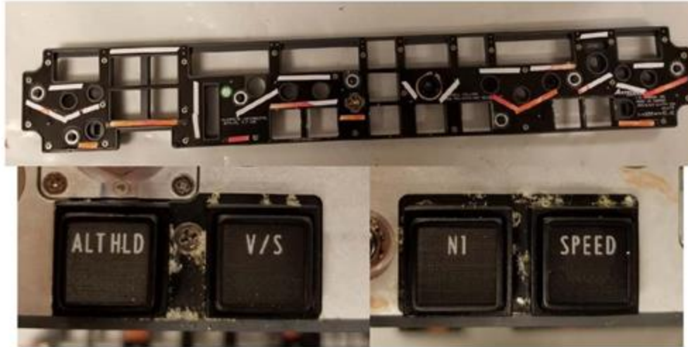
Figure 57. Top: Photo of the reverse side of [REDACTED] MCP light plate showing red fluid indicator tape, evidence of fluid intrusion. Lower Left and Right: Photos of the front of the MCP housing with light plate removed, showing a whitish powdery substance, likely corrosion product.
