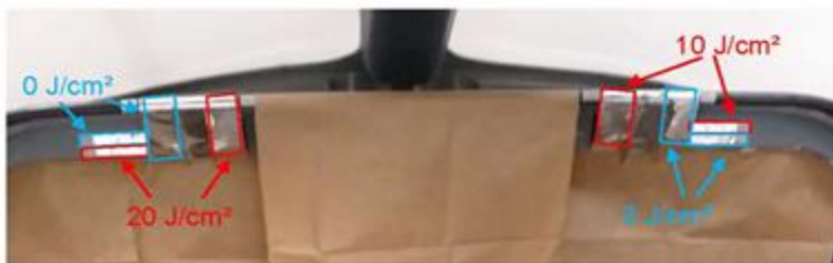
Figure 8 – Test 2 setup – Energy zones identification
