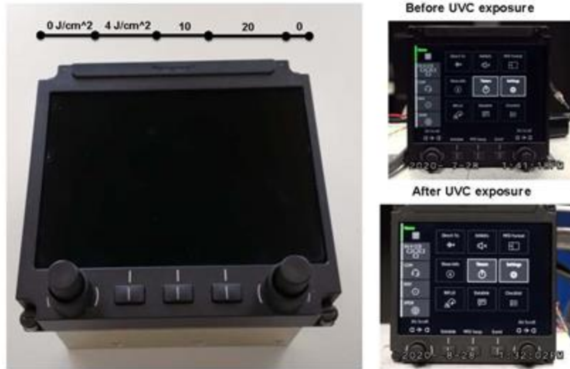
Figure 25: TSC 2.0 cockpit touchscreen display. Left: UV progressive doses; Right: Before and after display.
