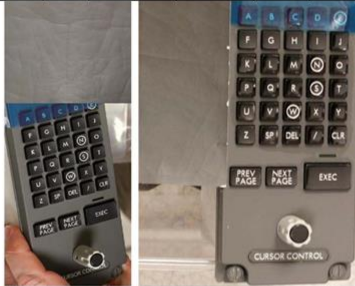
Figure 6: ■ gray color scheme; initial (left), after 16 cycles of Sani-Cide EX3 (right)
