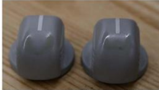
Figure 11: Calla 1452 remaining on knobs of P5-13 panel after 10 -12 minute dwell time
