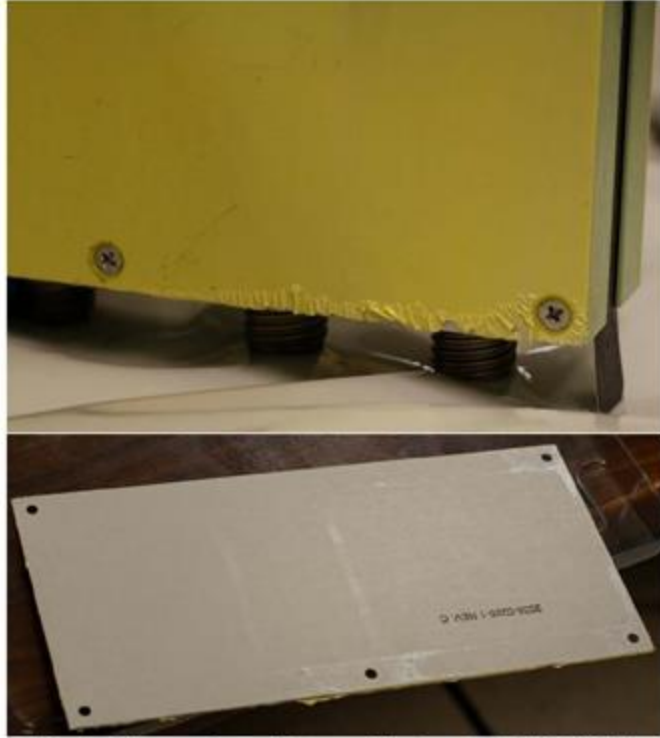
Figure A-1: Primer adhesion failure on flap module assembly due to Sani-Cide EX3 dripping down the side of the assembly (see SR17024 for additional details)
