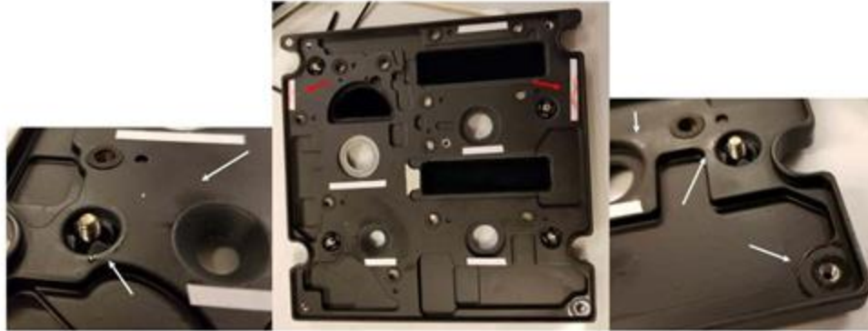
Figure 34. Photos of the [REDACTED] P5-6 Cabin Pressure Selector Panel display plate after 130 applications of Calla 1452. Wet residue (white arrows) was visible on some flat surfaces, around knob and switch holes and around fastener holes. Fluid ingress along the sides of the display plate was evidenced by red fluid detection tap (red arrows).
