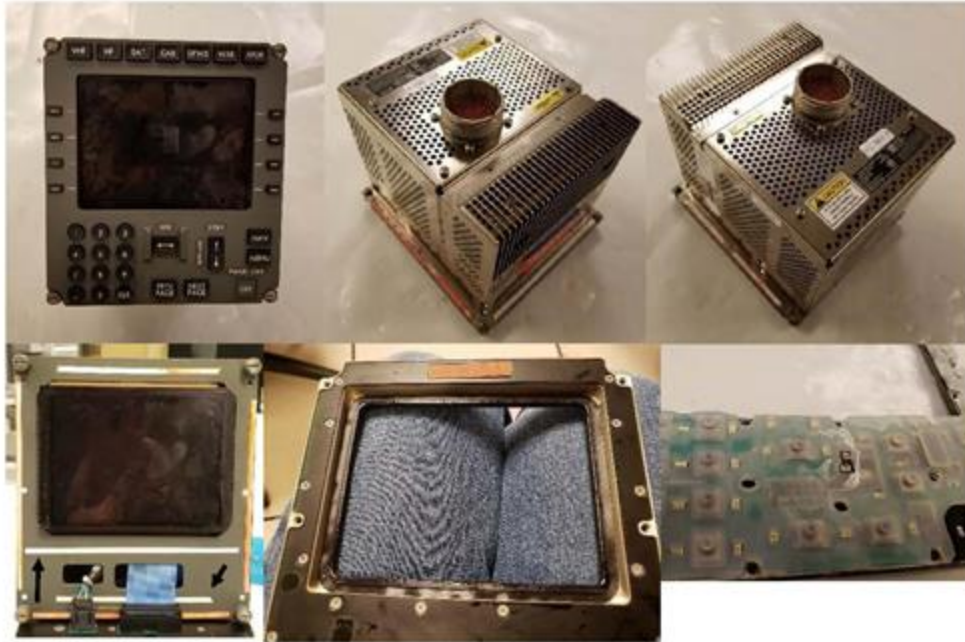
Figure 64. Photos showing condition of [REDACTED] TCP after 210 th application of Calla 1452. Top Row: External condition of the TCP. The red tape along the underside edges of the housing indicated fluid intrusion between the housing and mounting provisions. Bottom Left: Photo showing the front plate of the housing with light plate removed. The presence of red tape along the majority of the side edges indicated fluid intrusion, but the pristine white tape (black arrows) suggested that much of the fluid never penetrated significantly interior from the joint edges. Bottom Center: Photo of the reverse side of the light plate. Fluid and residue were evident along the edges of the display cutout, suggesting repetitive fluid intrusion and evaporation. Bottom Right: Photo of the rubber pad inside of the light plate. Whitish residue was present on surface, indicating repeated fluid intrusion.
