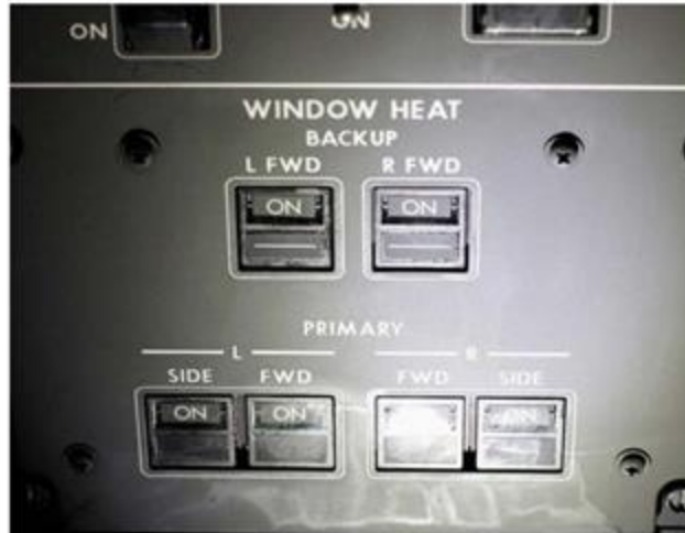
Figure 5: Example of sticky residue and streaks of dried Sani-Cide EX3 on surfaces from testing in a [REDACTED] flight deck
