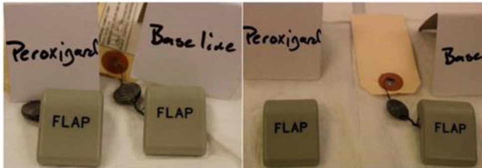
Figure 6: Gray "flap" knob; initial (left), after 50 cycles of Peroxi-gard (right)
