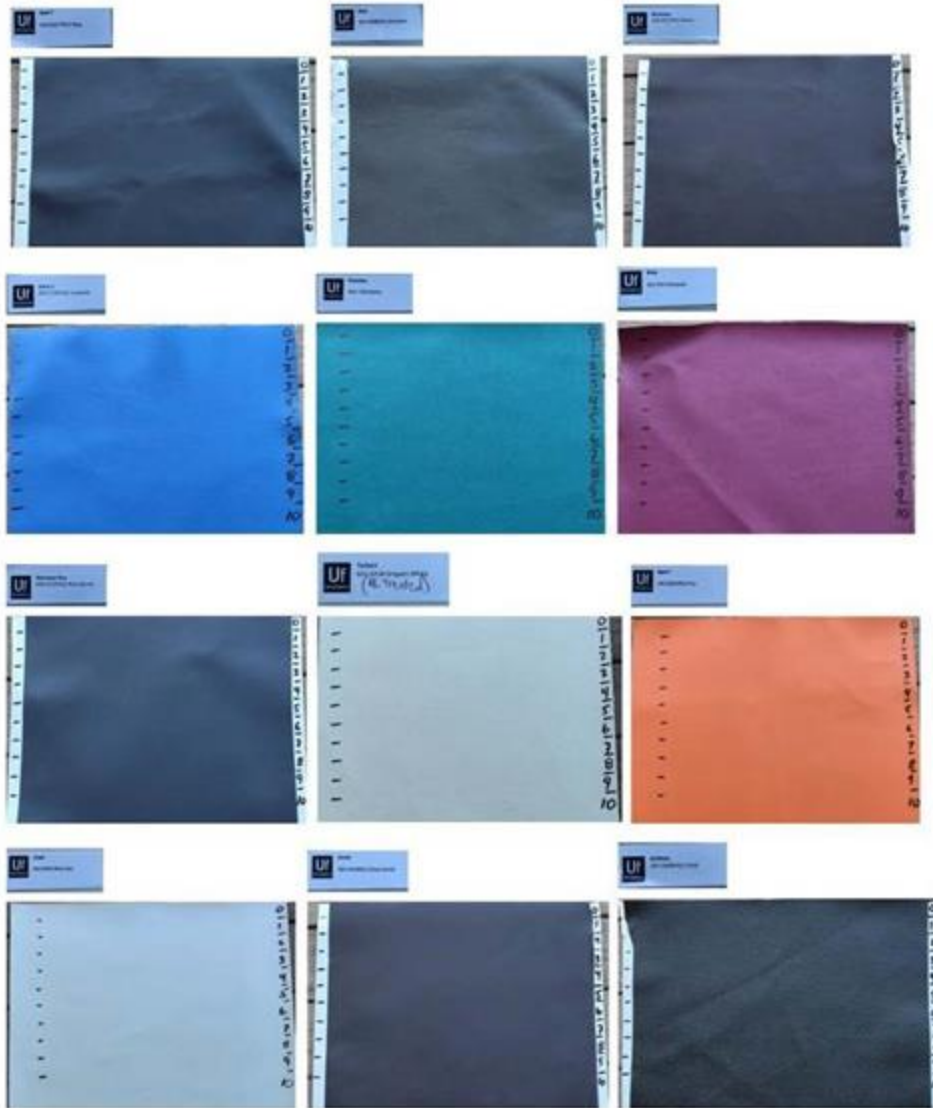
Figure 33. Ultrafabrics Samples, Progressive Exposure to 40 J/cm 2
