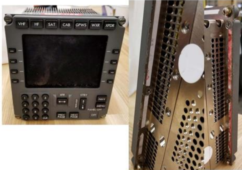
Figure 42. Left: Photo of [REDACTED] TCP after 130 applications of Calla 1452. Center and Right: Photos of the same LRU from the reverse, indicating fluid ingress between the undersides of the housing front plate and mounting provisions, as evidenced by red fluid intrusion tape.
