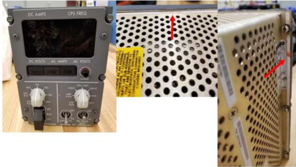
Figure 32. Left: Photo of P5-13 after 130 applications of Calla 1452. Residue was visible on the display screen. Center and Right: Photos of the same LRU, reverse side, indicating minor fluid ingress between the underside of the lip of the housing front plate and the mounting provisions, as evidenced by faint red fluid intrusion tape (red arrows).
