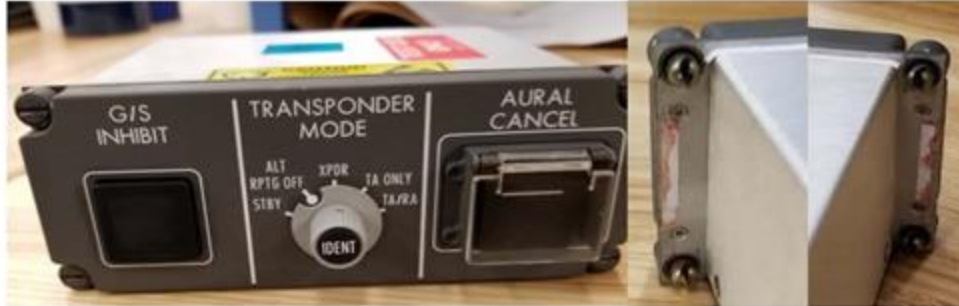
Figure 39. Left: Photo of [REDACTED] Alerting and Transponder Control after 130 applications of Calla 1452. Center and Right: Photos of the same LRU from the reverse, indicating fluid ingress between the underside of the housing and the mounting provisions, as evidenced by red fluid intrusion tape.
