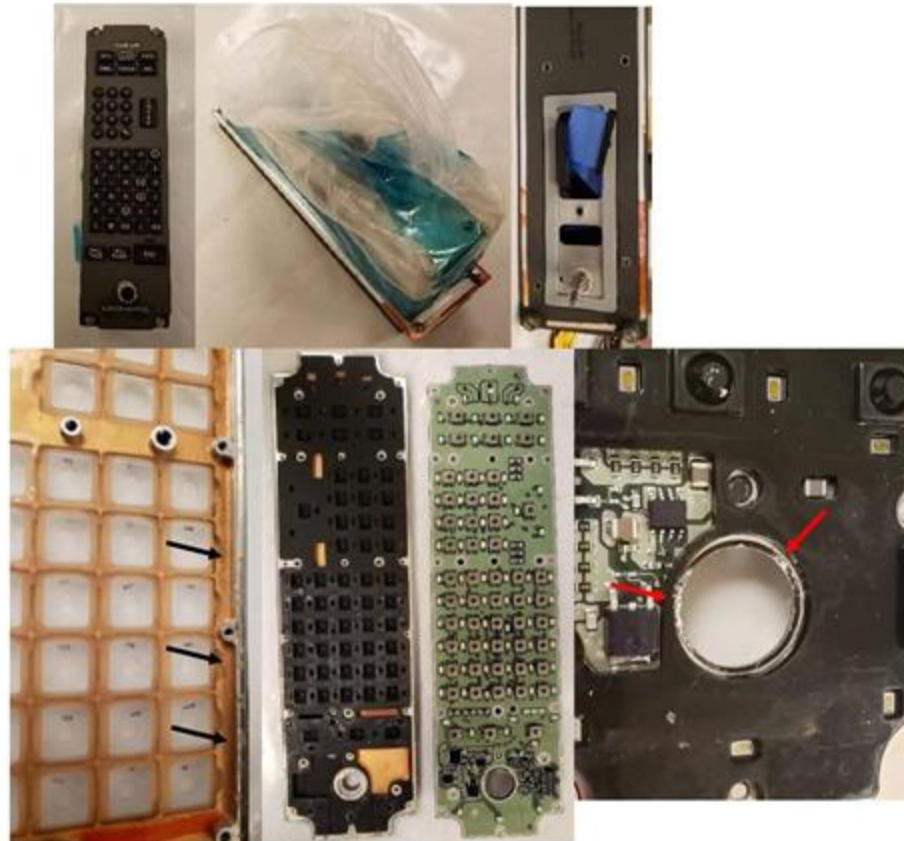
Figure 59. Photos showing condition of [REDACTED] MKP after 210 th application of Calla 1452. Top Left and Top Center: Exterior condition of the MKP after spray; red tape on the reverse side of the housing lip indicated fluid ingress between the housing and mounting provisions of the test rig. Top Right: Forward face of the housing with red tape along the lower side edges indicated fluid ingress between the housing and light plate. Bottom Left: Residue (black arrows) was present along the inside corner of the reverse side of the light plate front plate, indicative of repetitive fluid intrusion and evaporation. Bottom Center: Residue was present along portions (white circle) of the rubber pad and suggests fluid contact with the mating printed wiring board surface. Bottom Right: White powder (red arrows), likely corrosion product, was present along the edge of the cutout for the dial. Also, faint whitish residue traces were present on much of the rubber pad surface.
