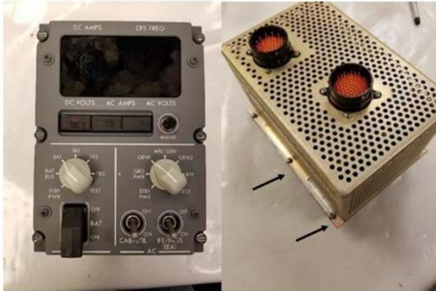
Figure 48. Photos showing external condition of [REDACTED] P5-13 panel after 210 th application of Calla 1452. The indicator tape has turned red (black arrows) along an edge of the back side of the housing lip, indicating the presence of relatively small quantities of fluid ingress between the panel housing and the mounting provisions.
