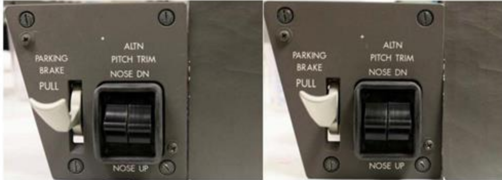
Figure 10: █ gray color scheme; initial (left), after 20 cycles of Calla 1452 (right)
