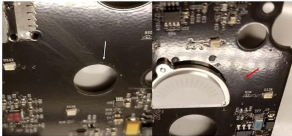
Figure 35. Photos of the [REDACTED] P5-6 Cabin Pressure Selector Panel display plate printed wiring board after 130 applications of Calla 1452. Residue (white arrow) was visible around the selector knob cutout. An evaporate trail (red arrow) was visible on the conformal coating near the semicircular LED display. These features were not thought to be direct contributors of the observed inoperative switch.
