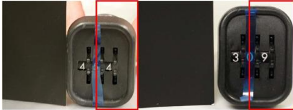
Figure 9: [redacted] black color scheme; initial (left), after 16 cycles of Sani-Cide EX3 (right)
