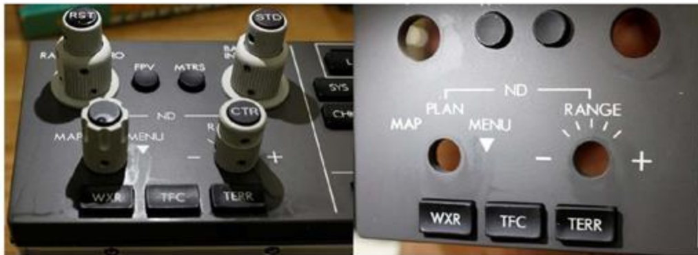
Figure 20: Indications of Calla 1452 dripping and residue on ██████ DCP
