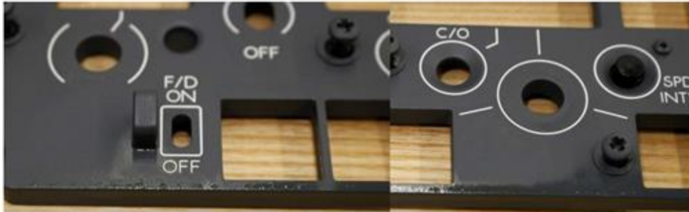
Figure 18: Calla 1452 residue and pooling along bottom edge of MCP light plate
