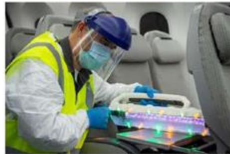
Figure 5: Kr/Cl 222 nm excimer lamp in [redacted] Far-UV 222nm mobile wand prototype.
