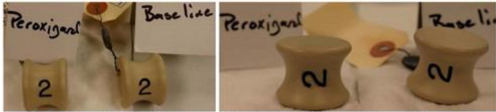
Figure 3: Tan numbered knob; initial (left), after 50 cycles of Peroxi-gard (right)
