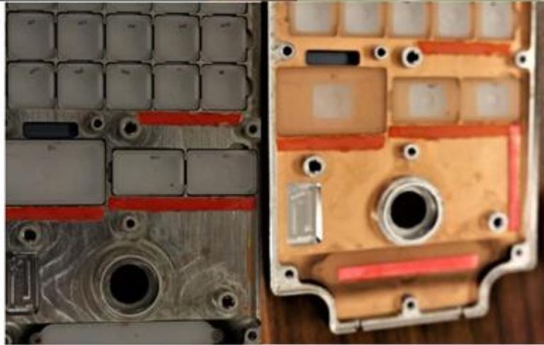
Figure 27: Indications of ingress and corrosion in MKP assembly
