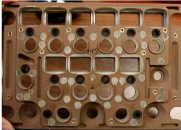
Figure 5: Back of ACP light plate showing no signs of ingress or corrosion
