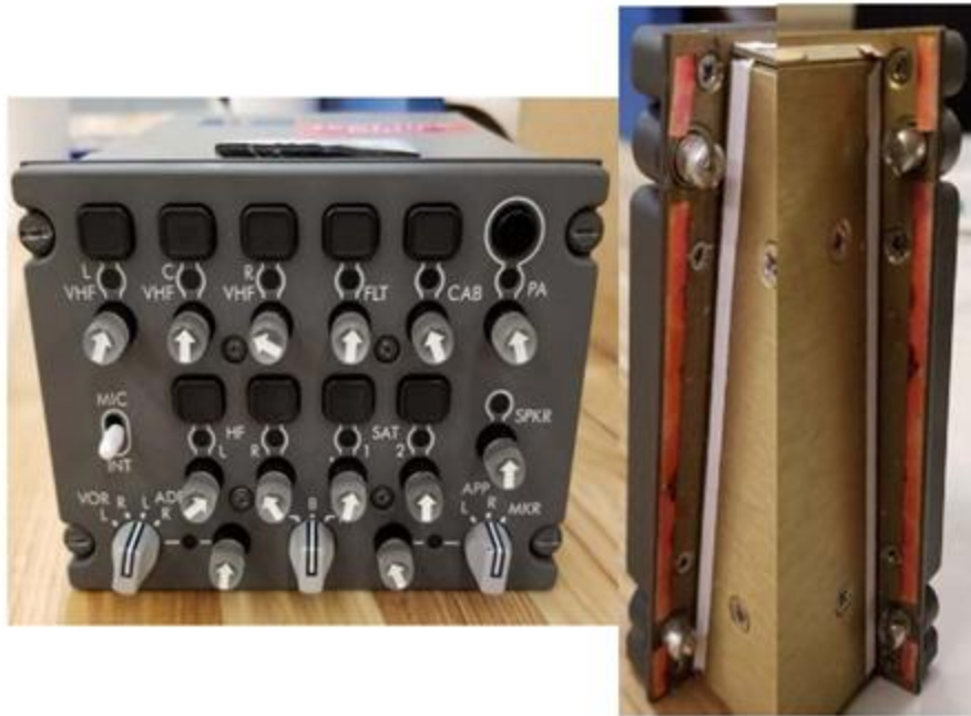
Figure 41. Left: Photo of [REDACTED] ACP after 130 applications of Calla 1452. Center and Right: Photos of the same LRU from the reverse, indicating fluid ingress between the undersides of the housing front plate and mounting provisions, as evidenced by red fluid intrusion tape.
