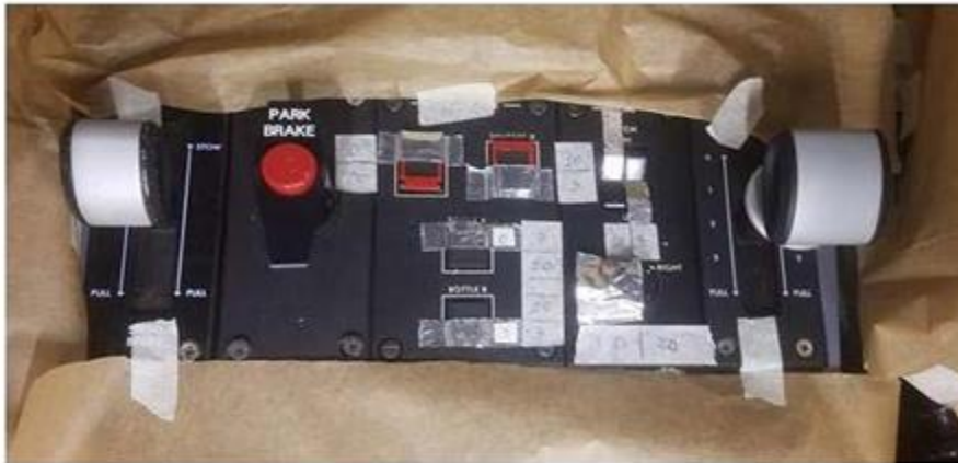
Figure 6 - Components from test 1 after 17J/cm 2 of energy applied
