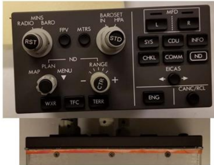
Figure 44. Top: Photo of [REDACTED] DCP after 130 applications of Calla 1452. Bottom: Photo of the same LRU from bottom side, indicating fluid ingress between the housing and mounting provisions, as evidenced by red fluid intrusion tape.
