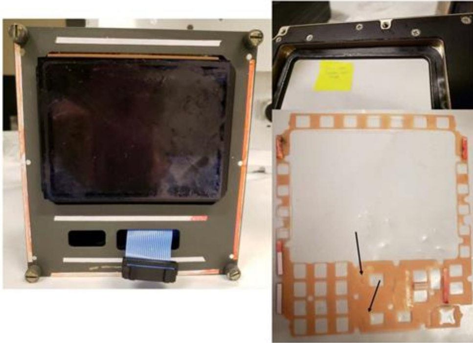
Figure 43. Left: Photo of [REDACTED] TCP after 130 applications of Calla 1452 with light plate removed. Red fluid intrusion tap indicated the extent of fluid ingress between the light plate and the front plate of the housing. Top Right: Photo of the light plate reverse side, showing wet residue along the joint common to the light plate housing and along the cut for the display screen. Bottom Right: Photo of the light diffuser showing dimple marks (black arrows) due to previous misassembly (see Phase III.3 Results), and a likely contributor to button sticking.
