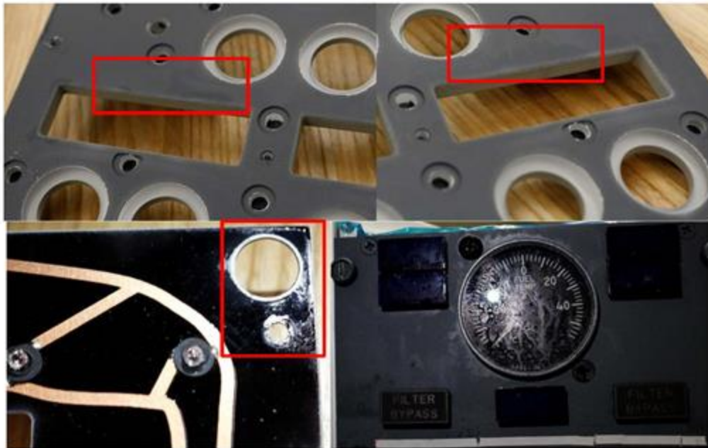
Figure 12: Moisture and residue observed on fuel control panel components
