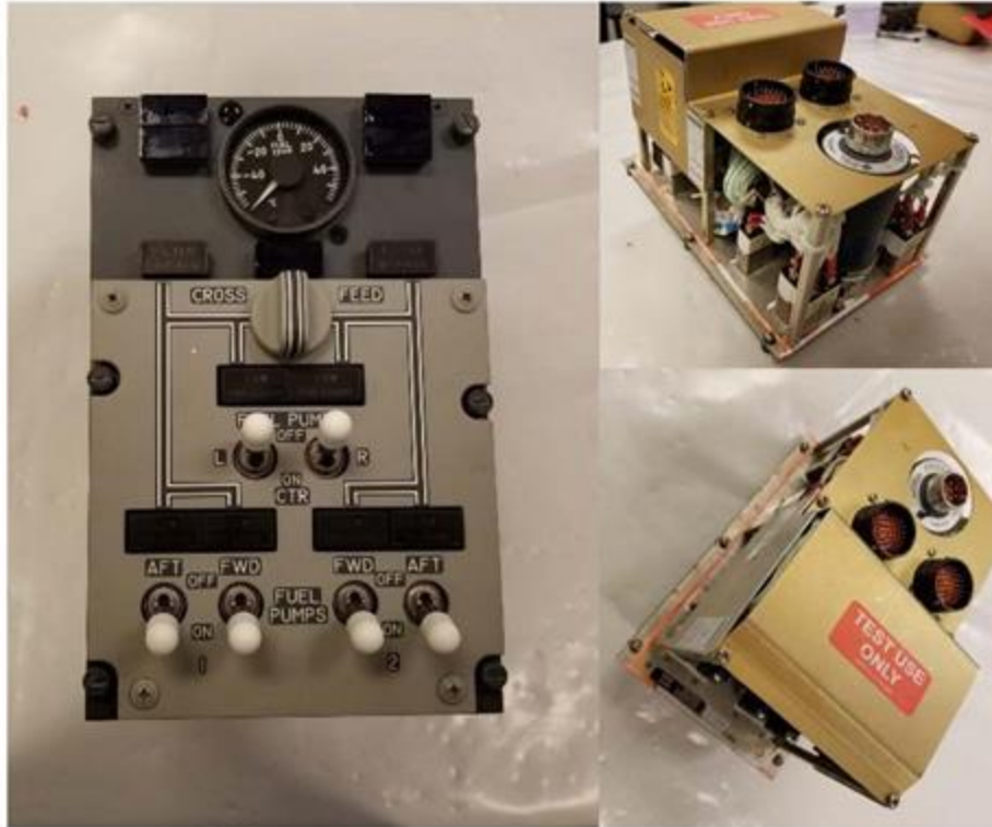
Figure 53. Photos showing external condition of Fuel Control Panel after 210 th application of Calla 1452. The indicator tape was red along several edges of the back side of the housing front plate, indicating the presence of relatively large quantities of fluid ingress between the panel front plate and the mounting provisions.
