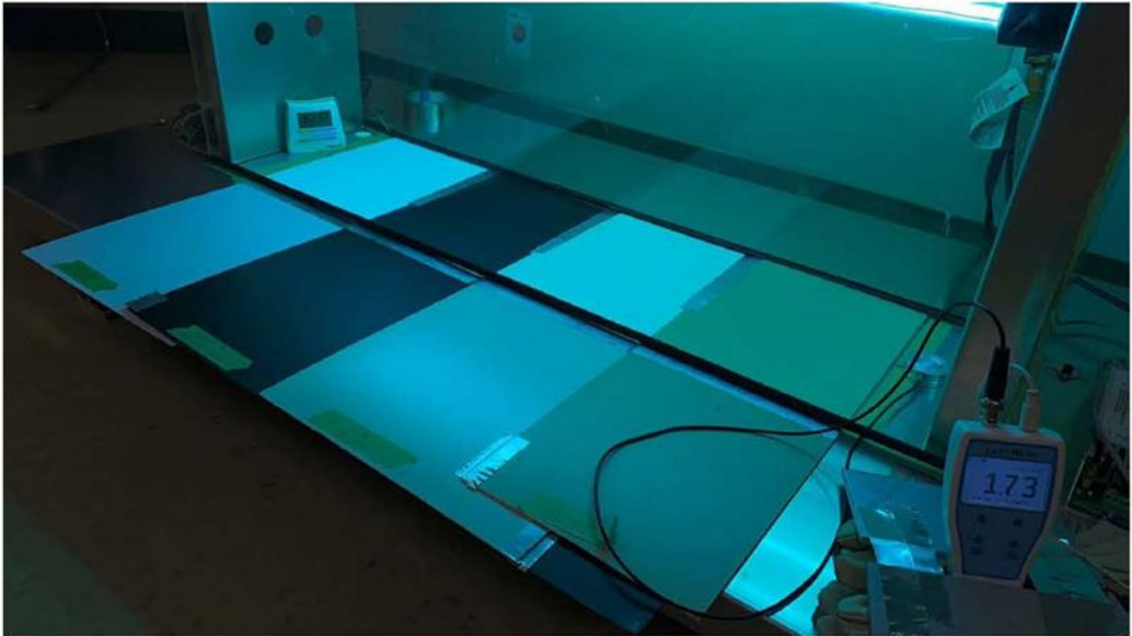
Figure 4 – Image of Set 1 with half of each material inside the acrylic cover with UVC lights and the remaining half not exposed to UVC. This image was captured on December 10, 2020 at 14:40 showing a reference reading of 1.73mW/cm 2 . Correcting this by the 0.7295 factor results in 254nm irradiance of 2.37 mW/cm 2 .
