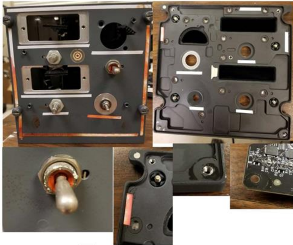
Figure 52. Additional photos of [REDACTED] P5-6 Cabin Pressure Selector Panel during disassembly. Upper Left: Photo of same LRU with display plate removed, revealing significant amounts of fluid were present between the housing front plate and the display plate, as evidenced by red indicating tape. Bottom Left: Close-up of manual control switch with white powder, likely corrosion product. Upper Right: Photo of the inside surface of the display plate with printed wiring board removed. Fluid was present around most corner inserts, and residue from previous exposure cycles remained. Bottom Center Photos: Close-ups of the red indicator tape and fluid residue around insert in corner. Lower Right: Photo of the display plate printed wiring board with fluid around the fastener hole.
