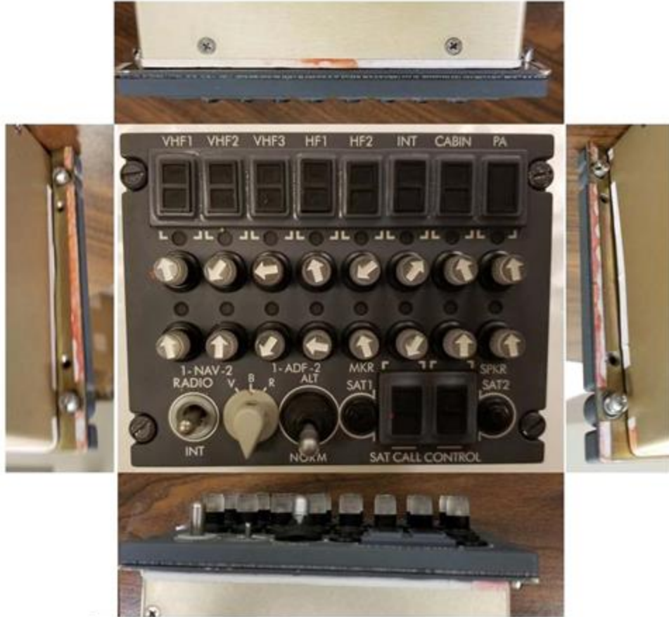
Figure 46. Photos of [REDACTED] ACP after 210 applications of Calla 1452. Photos indicate fluid ingress between the housing and mounting provisions, as evidenced by red fluid intrusion tape (photos taken after removal of light plate mounting screws).
