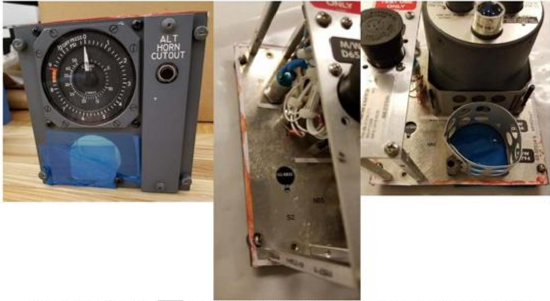
Figure 37. Left: Photo of the [REDACTED] Cabin Altimeter - Differential Pressure Indicator after 130 applications of Calla 1452. Center and Right: Photos of the same LRU, reverse side, indicating fluid ingress between the undersides of the front plate and mounting provisions, as evidenced by red fluid intrusion tape.
