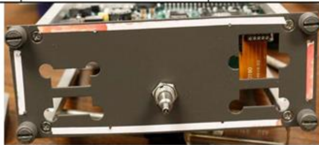
Figure 21: Minor indications of ingress on alerting and transponder control
