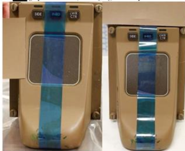
Figure 2: [redacted] brown color scheme; initial (left), after 20 cycles of 70% IPA (right)
