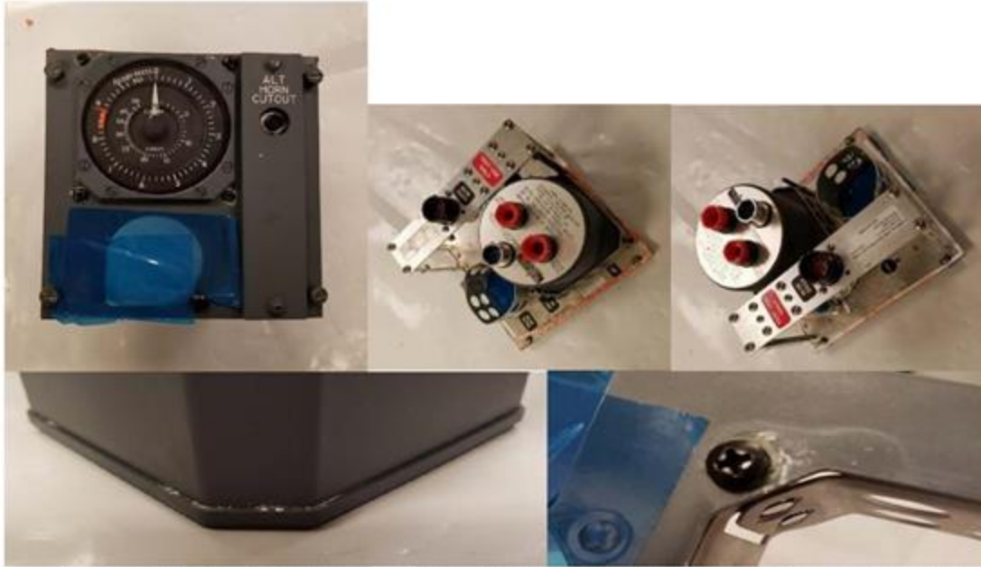
Figure 55. Photos showing condition of [REDACTED] Cabin Altimeter and Differential Pressure Indicator panel after 210 th application of Calla 1452. The indicator tape has turned red along several edges of the reverse side of the front plate, indicating the presence of relatively large quantities of fluid ingress between the front plate and the panel mounting provisions. The bottom photos show a white powdery substance emanating from under a fastener screw and along the joint of the altimeter canister faceplate.
