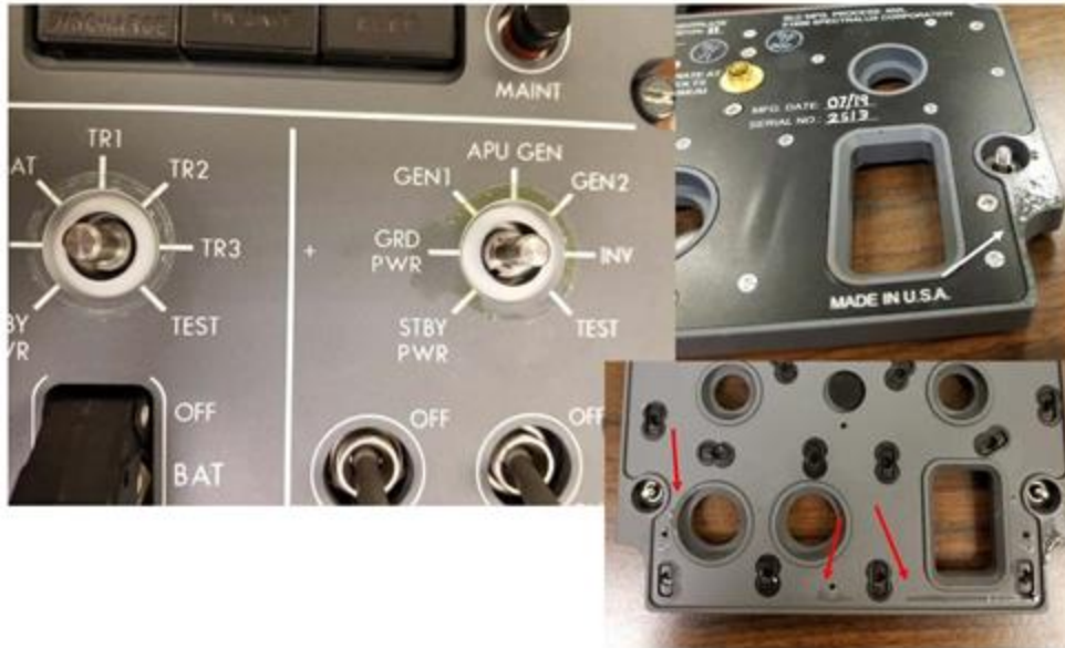
Figure 49. Photos showing condition of [REDACTED] P5-13 panel during disassembly after 210 th application of Calla 1452. Left: Fluid residue was present between both knobs and the light plate. Upper Right: Fluid (white arrow) was present on the reverse side of the light plate. Lower Right: Fluid (red arrows) was present on the reverse side of the light plate, between the light plate and printed wiring board (not shown).
