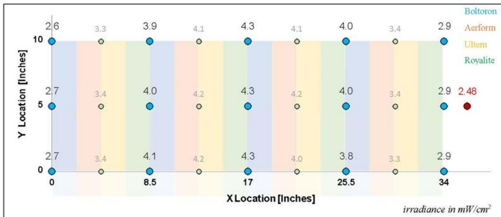
Figure 7 – The graph above shows the corrected irradiance measurements taken during Set 3. The material placement on the testbed is overlaid on the same graph to show the materials used during Set 3a. Measured values are shown in blue. Interpolated values are shown in green to facilitate calculation. The values show the steady state values in irradiance after the test chamber was allowed to reach a stable temperature and humidity.
