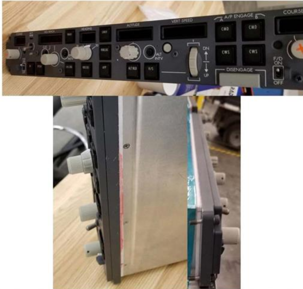
Figure 38. Top: Photo of [REDACTED] Mode Control Panel after 130 applications of Calla 1452. Bottom Row: Photos of the same LRU from the top and bottom sides, indicating minor fluid ingress between the underside of the housing and the mounting provisions, as evidenced by red fluid intrusion tape.
