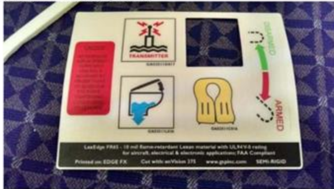
Figure 31. Colored Label Sample, After Exposure
