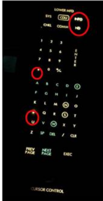
Figure A-3: Variance in backlight brightness in MKP (buttons with blue tint were covered with blue flash tape)
