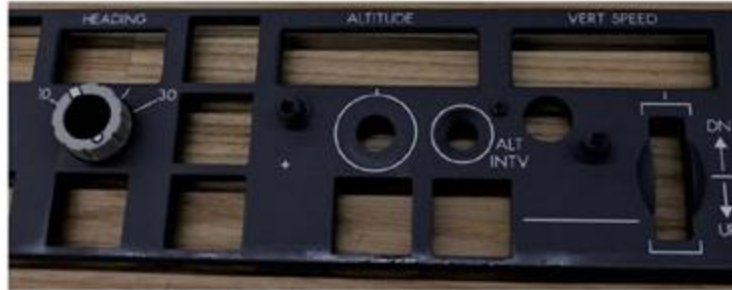
Figure 13: Calla 1452 remaining along bottom edge of MCP light plate after 10 _ 12 minute dwell time
