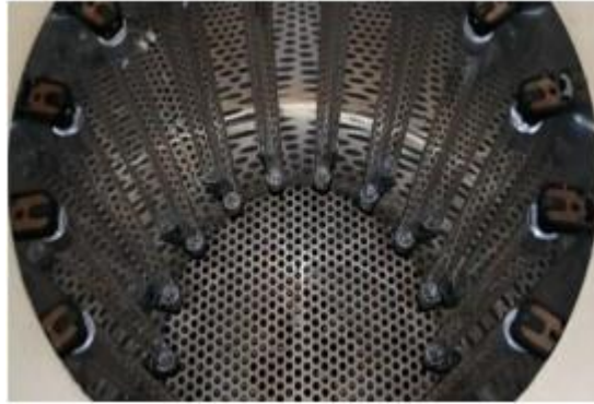
Figure 7. Reactor used for UV-C exposures
