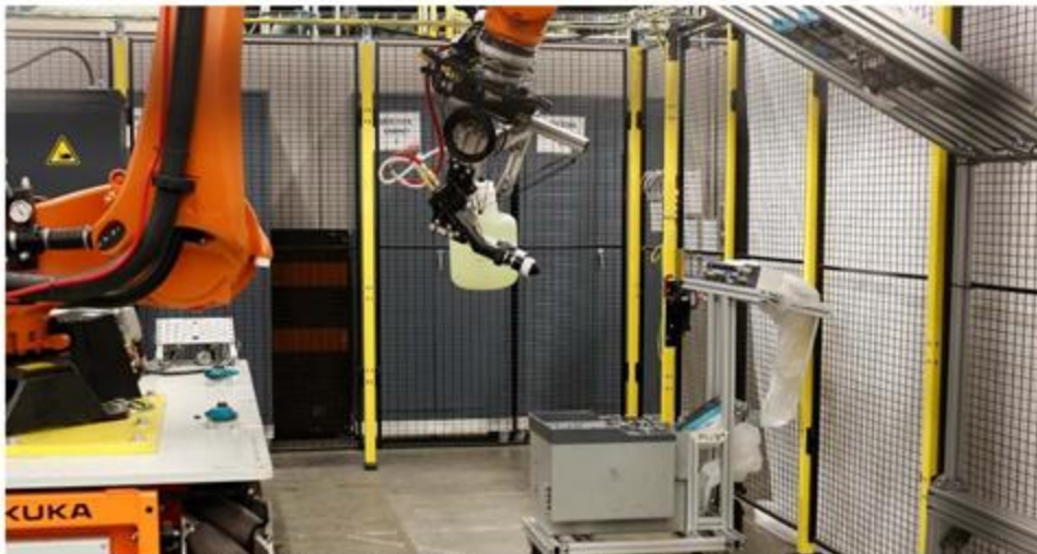
Figure 3: Setup of Calla 1452 e-spray testing using Kuka robot
