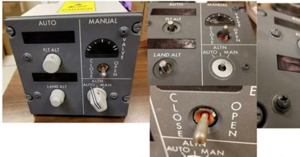
Figure 51. Left: Photo showing external condition of P5-6 Cabin Pressure Selector Panel after 210 th application of Calla 1452. None of the indicator tape applied externally had turned red (not shown). Upper Center: Photo of same LRU with knobs removed. Rings of fluid residue were present under all knobs. Lower Center: Photo of manual control switch exhibiting a white powdery substance, consistent with corrosion product. Right: Photo of loosened display plate attachment screws, showing a white powdery substance coincident with a shim or washer under the fastener head.
