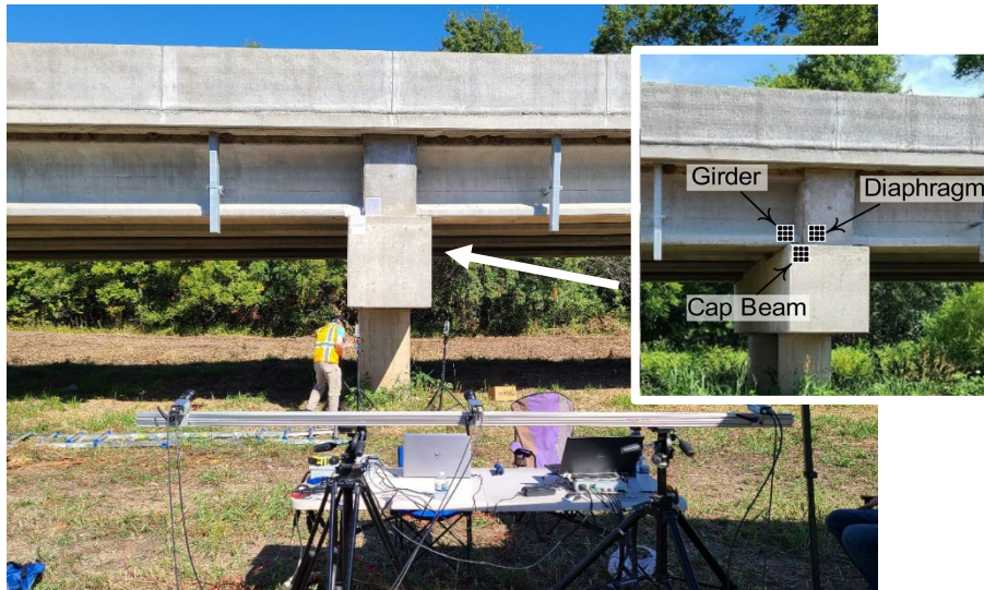
Figure 4-5. DIC camera setup and target locations
