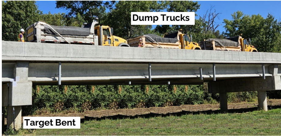
Figure 4-2. Loading span 3-4 with dump trucks
