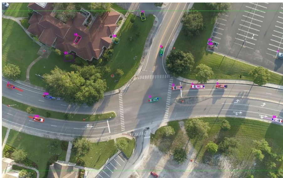
Figure 3.3 Vehicle tracking and trajectory extraction
