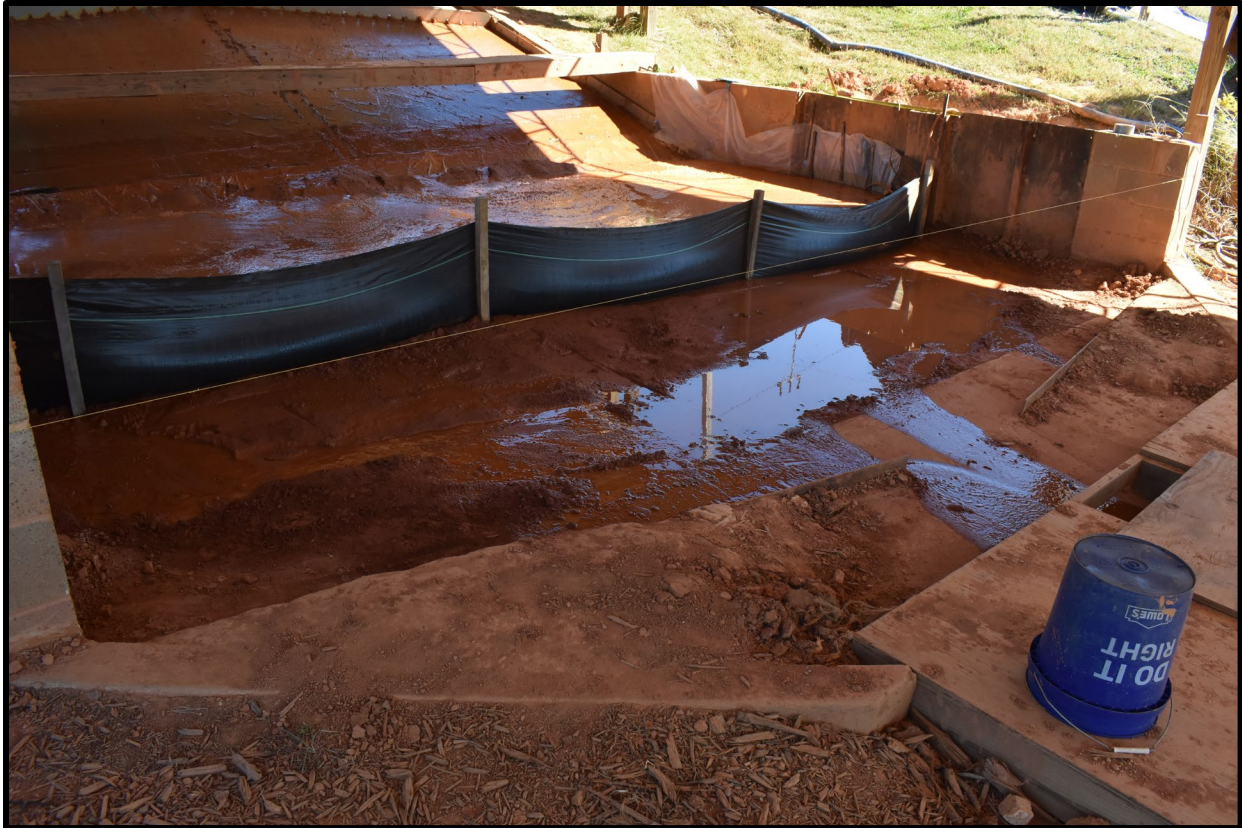
Figure 3.14 Reduced Sagging Experienced by M2
