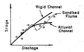
This stage-discharge relation helps identify not only the stage relative sto discharge but the effects of different roughness elements and flow required on the stage-discharge relation
