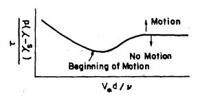
Shields' diagram; determines the critical shear stress defining beginning of motion of particles ( $\tau_c$  is widely used in transport equations) and can be used to establish a design procedure for stabilizing the bed and banks of mineral banks of rivers
