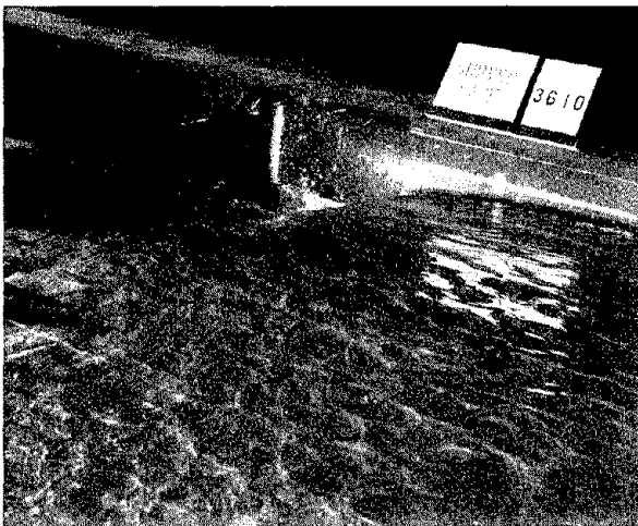
Figure 7-6. - 3.0 ft by 4.0 ft (0.91 m by 1.22 m) CV - 3-1/4 - 4-1/4 sump grate at three flow depths, Z = 16 .
