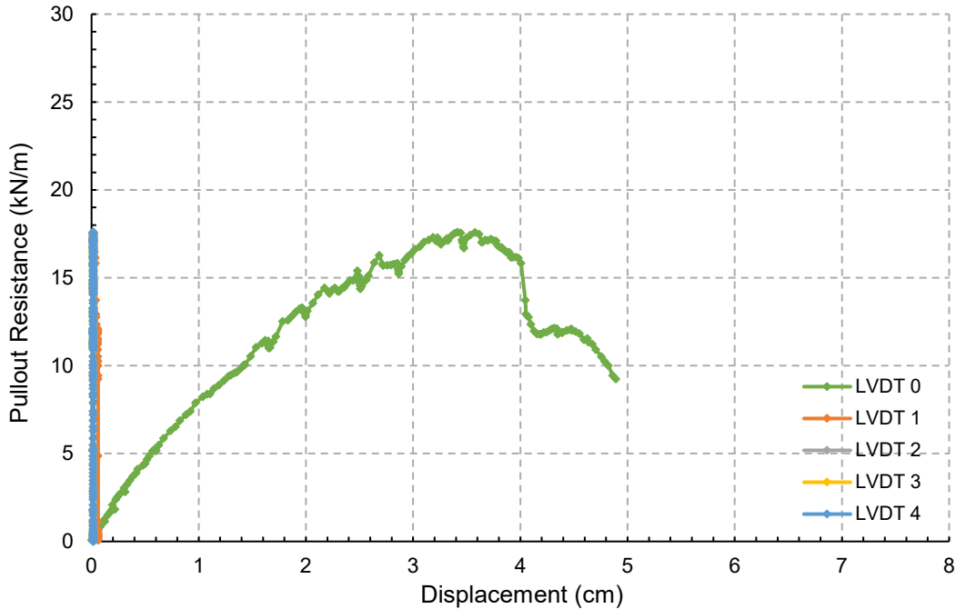
Figure 5.56 GT reinforced clay at 38 kPa
