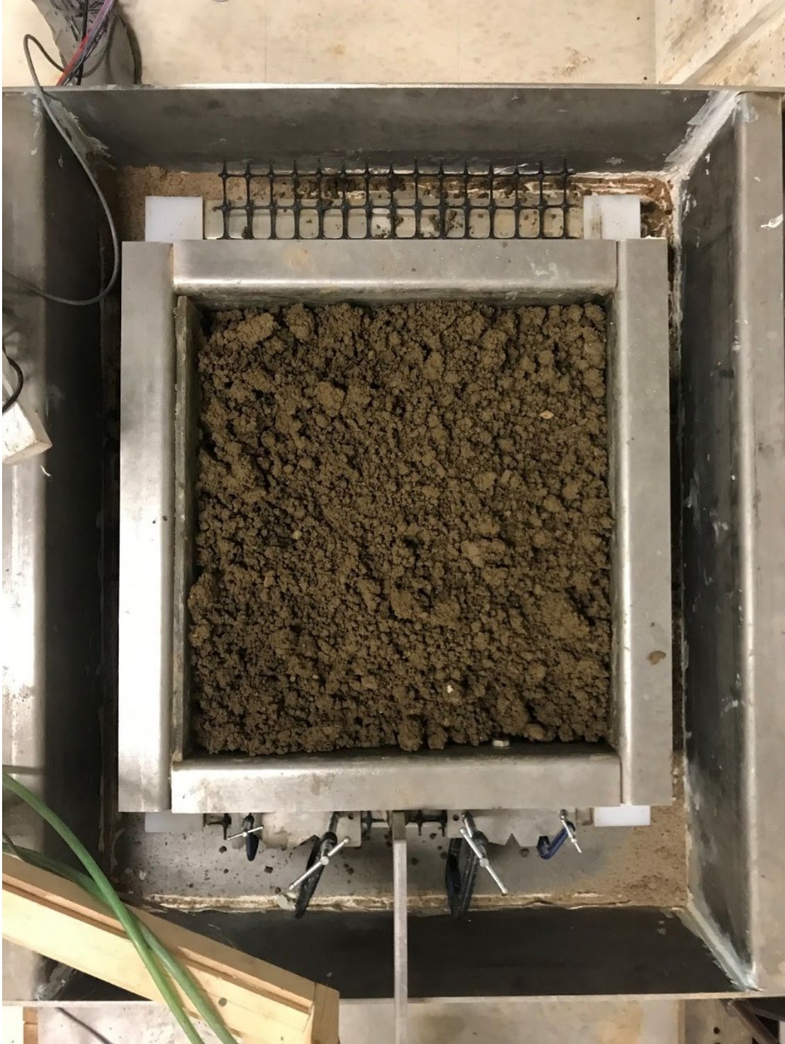
Figure A.2 Installation of geosynthetic specimen in silt
