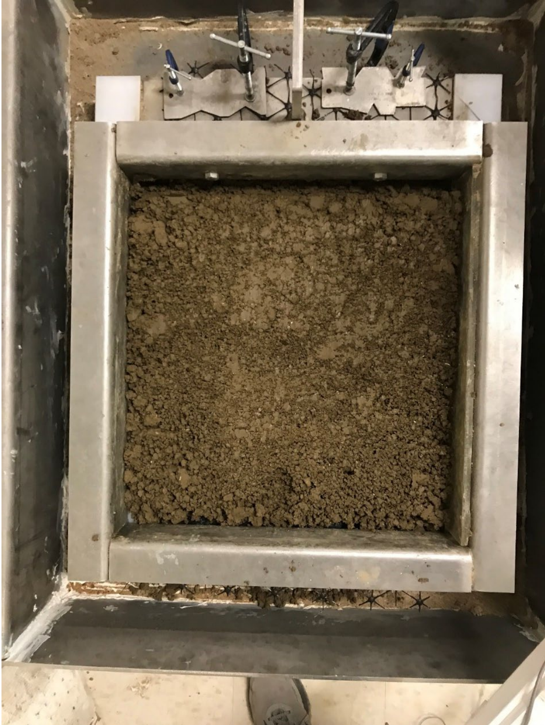
Figure A.4 Surface of compacted soil in the box
