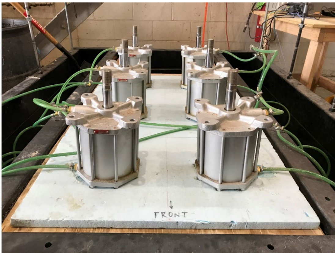
Figure 4.12 Pneumatic pistons used to apply the confinement pressure over the tested sample
