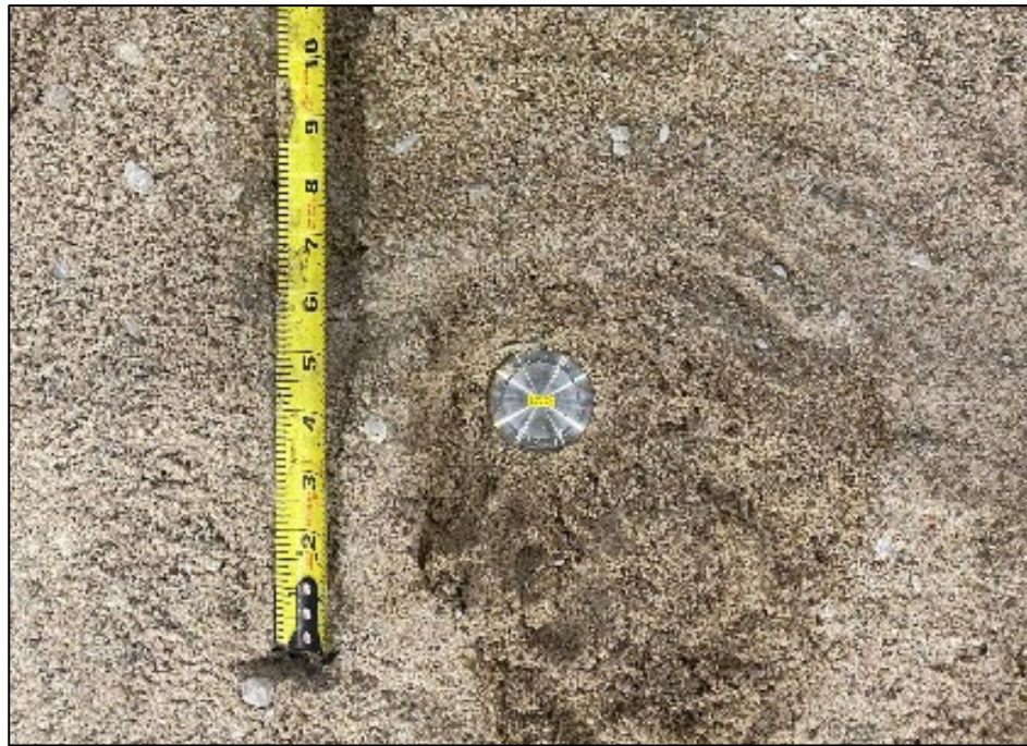
Figure 4.39 Pressure cell on compacted sand layer
