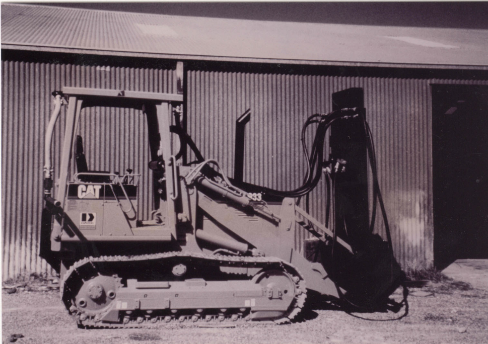
Figure 24. Hydraulic Crawler Rig for Lime Injection.
