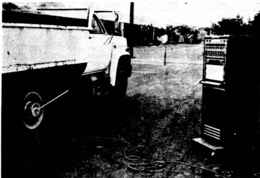
(b) Installed on truck for functional dynamic test
