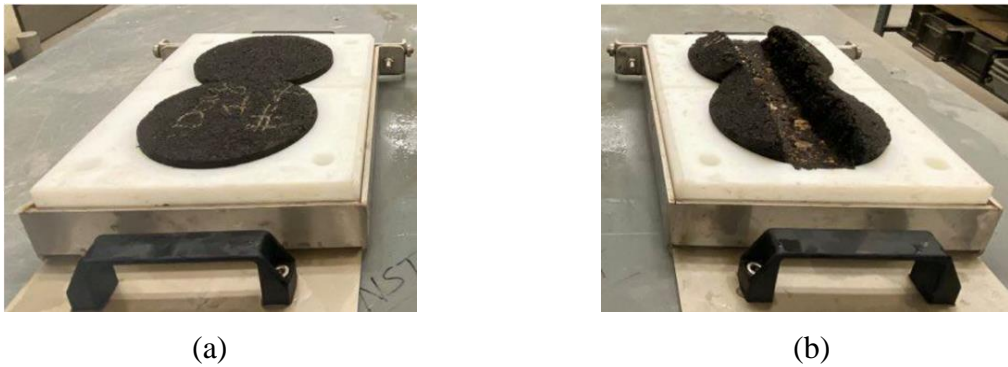
Figure 3.3 HWTT test specimens, (a) before testing and (b) after testing.
