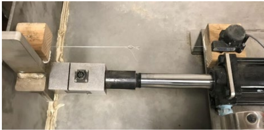
Figure 3.9 The horizontal LVDT.
