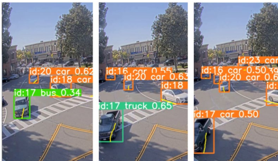
Figure 2.4 Example of an object changing classification from bus to truck to car.
