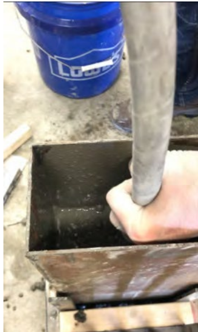
Figure 3.12 Insertion of the vibrator in L-box
