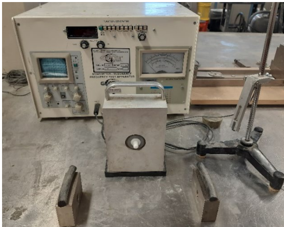
Figure 3.28 F-T resistance test setup with sonometer
