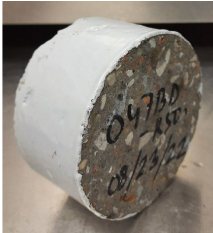
Figure 3.30 Saw-cut concrete specimen for rapid chloride penetration test
