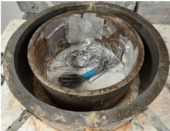
Figure 3.33 Restrained shrinkage test standard steel mold
