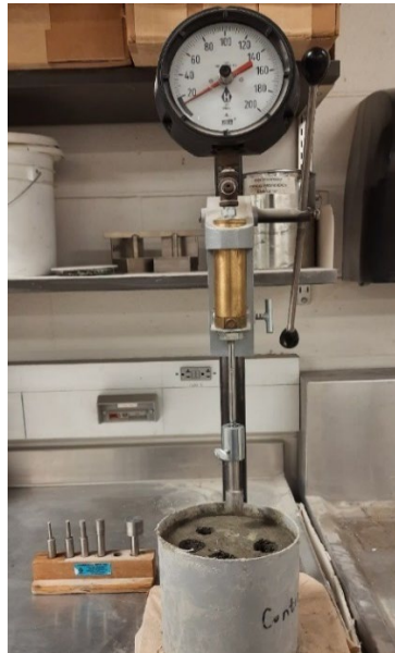
Figure 3.14 Penetration resistance test for concrete set time
