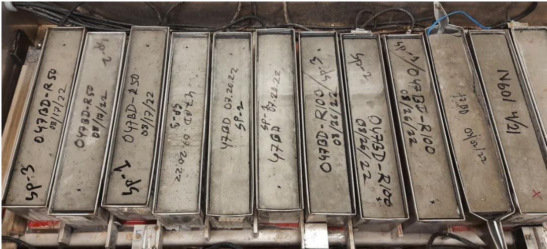
Figure 3.27 Concrete specimens in the freeze-thaw chamber
