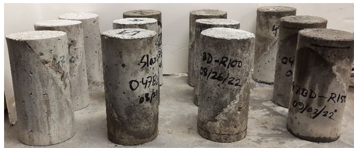
Figure 3.24 Slant shear specimens after casting
