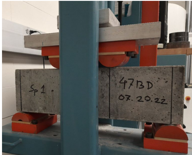
Figure 3.17 4-point bending flexural test setup
