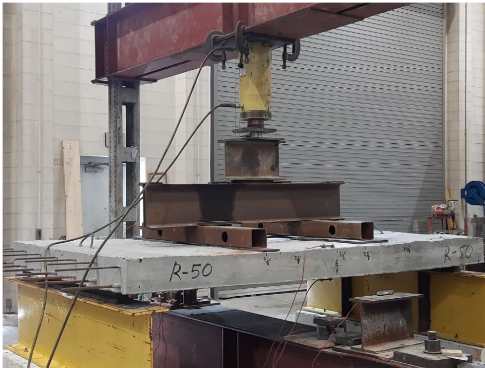
Figure 5.8 Flexure test setup and instrumentation
