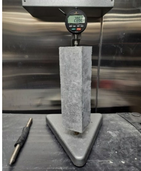
Figure 3.35 Change of concrete length measurement
