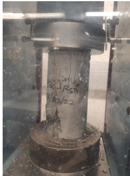
Figure 3.16 Compressive strength test setup
