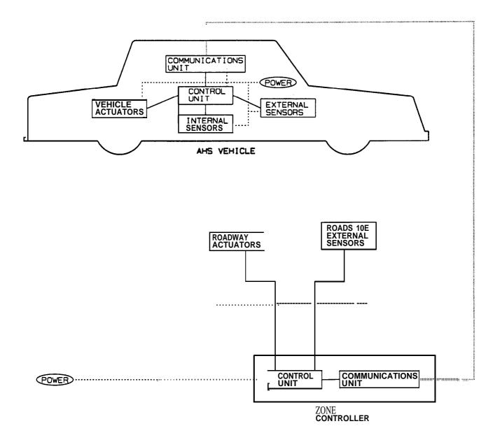
Figure 8. AI- R3systemarchitectu reschematic.
