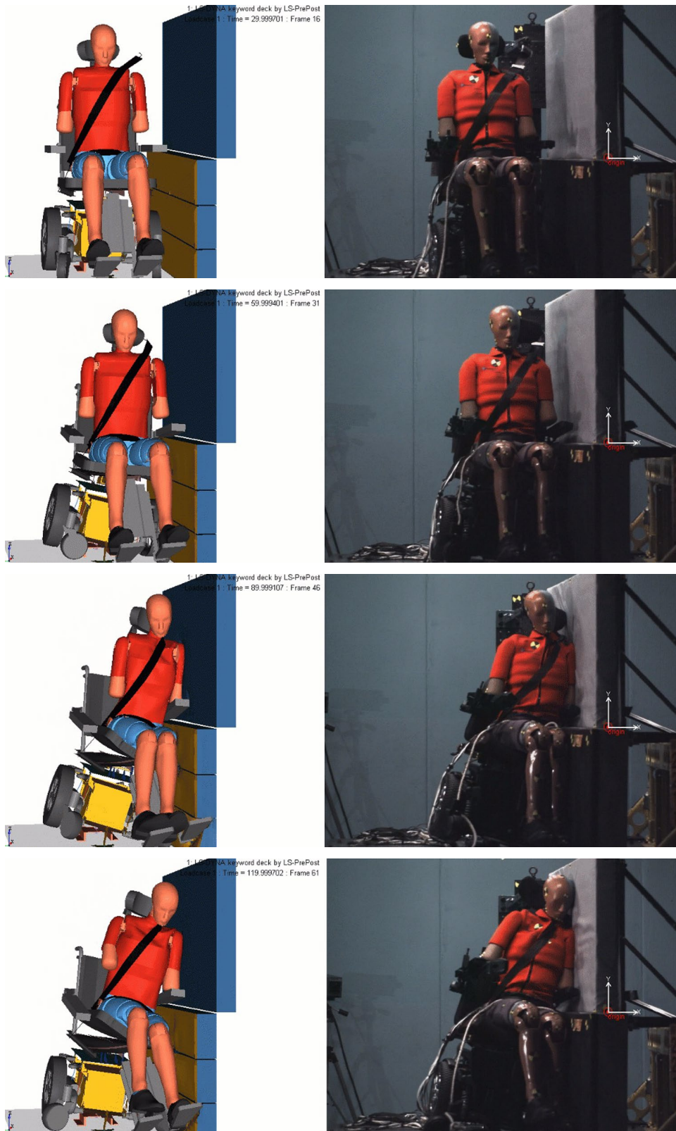
Figure C-10. Comparison of model and test kinematics for power wheelchair, secured by traditional docking, under nearside impact, at 30, 60, 90, 120 ms.
