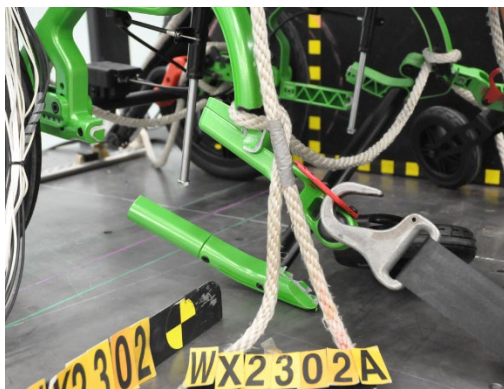
Figure 41. Component failure in nearside impact test of Leggero Enzo
