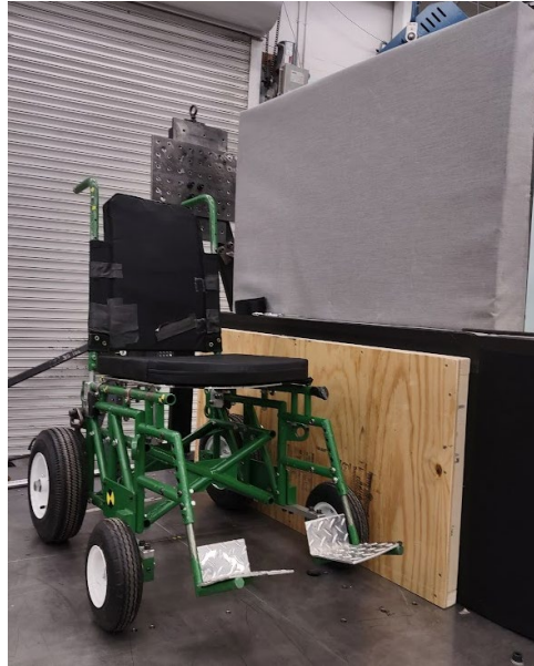
Figure 36. Updated wall and 50-mm thick positioning tool proposed for testing wheelchairs in nearside impact
