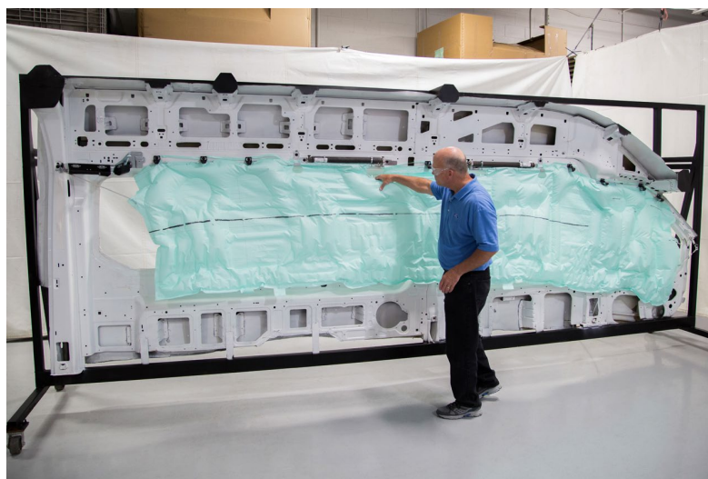
Figure 4. Testing of prototype curtain air bag using a body-in-white fixture
