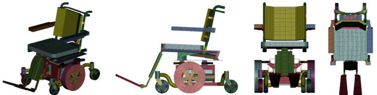
Figure C-2. CAD geometry used to create power wheelchair model
