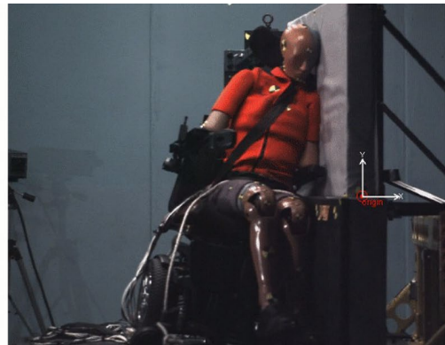
Figure 68. Peak excursion comparison of FE model of power wheelchair secured by traditional docking to test (WX2211) under nearside impact
