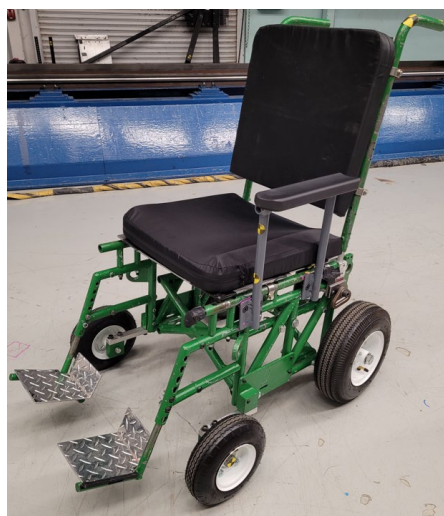
Figure B-2. Photo of the SWCSI, modified from the SWCB to include different wheels and attachment bolts, a shifted lap belt anchor location, a left armrest, and a contoured seat cushion
