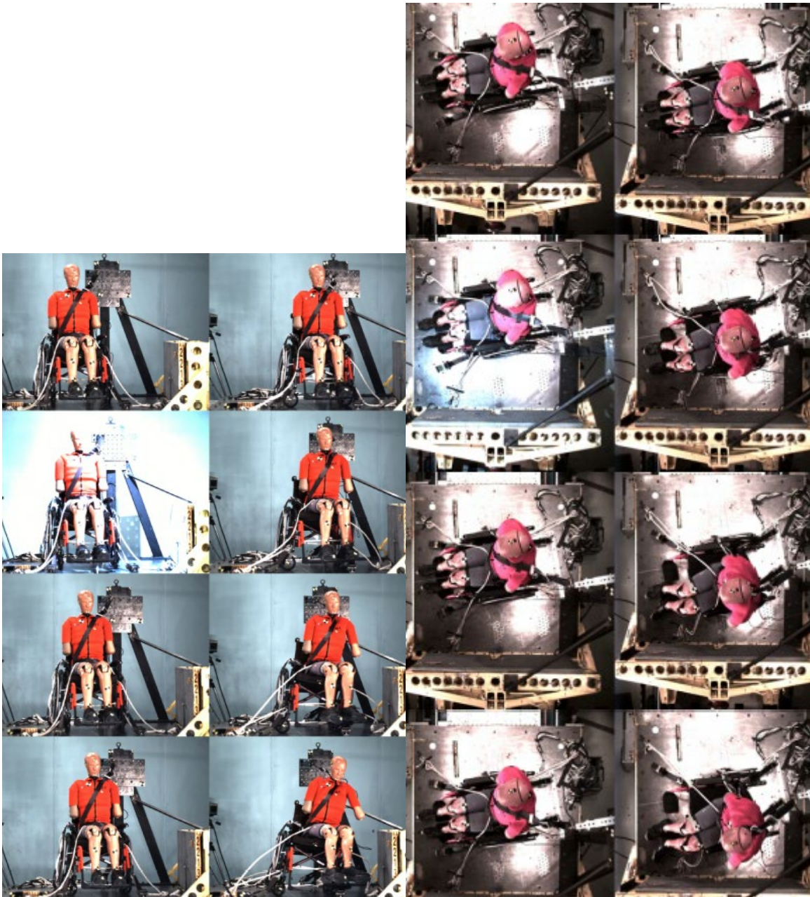
Figure F-7. Kinematics for WX2213, Ki Mobility+SWTORS, nearside (center) without wall, from -20 to 120 ms every 20 ms
