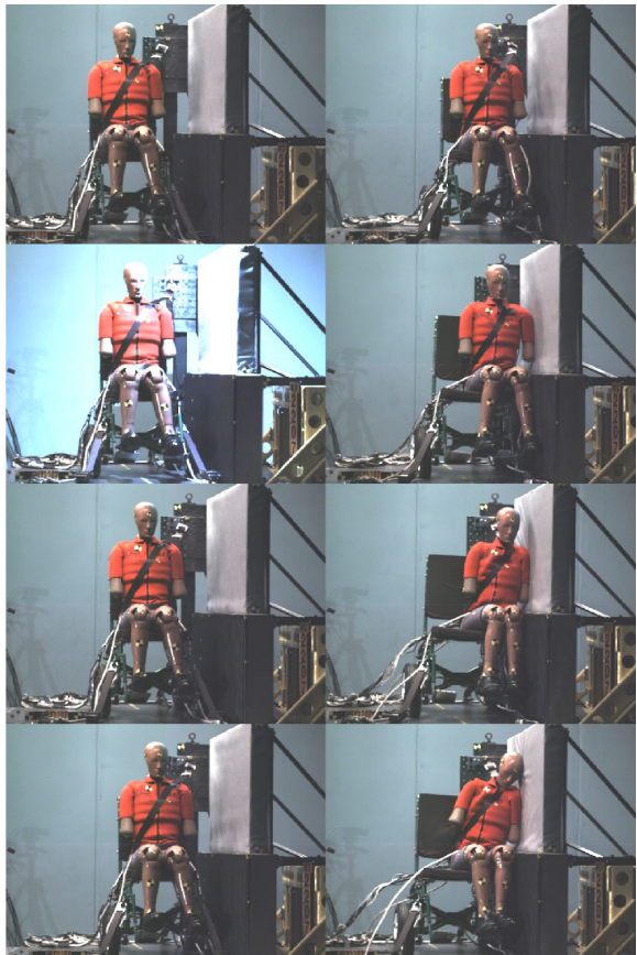
Figure F-5. Kinematics for WX2207, SWCB+SWTORS, nearside with wall, from -20 to 120 ms every 20 ms
