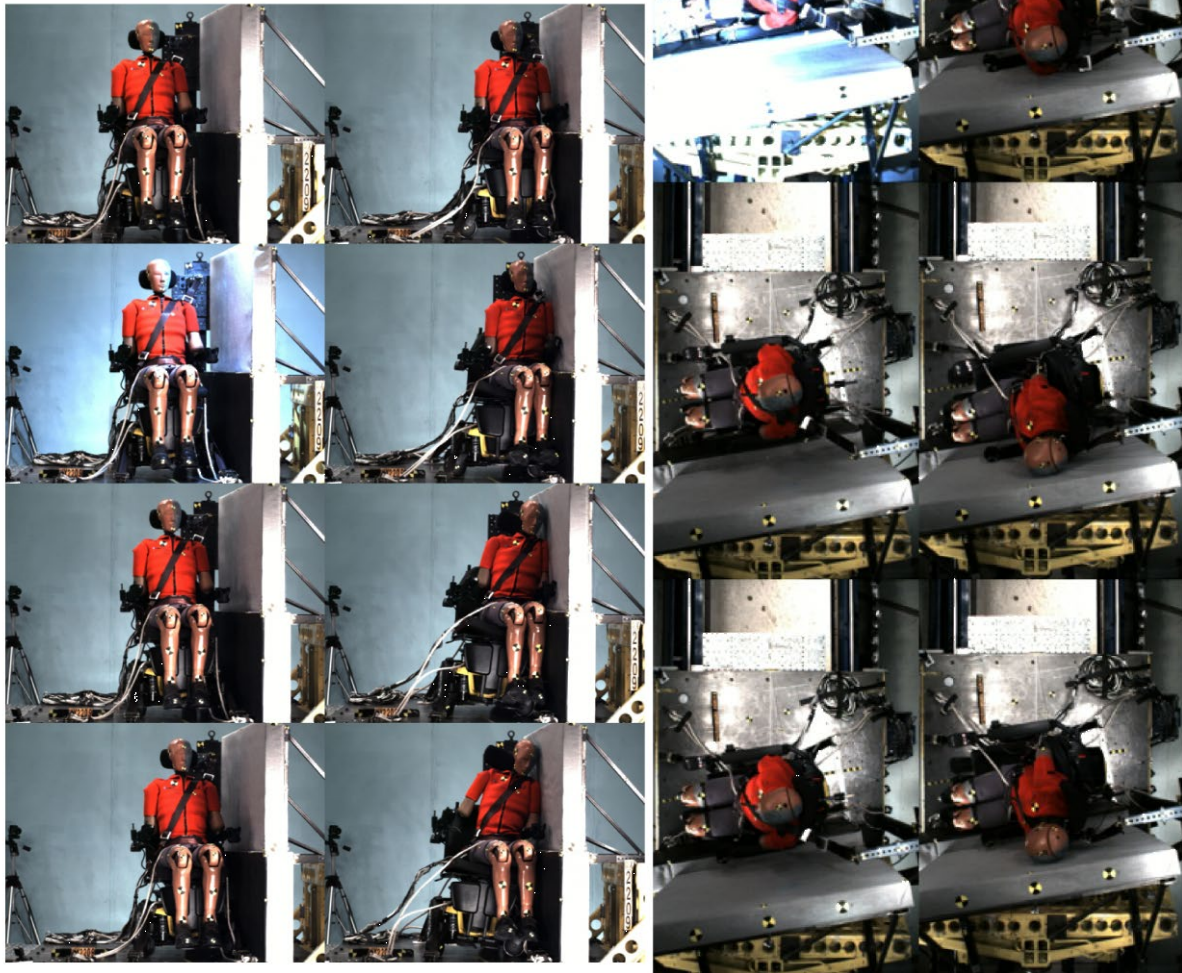
Figure F-4. Kinematics for WX2209, Quantum Edge+SWTORS , nearside with wall, from -20 to 120 ms every 20 ms
