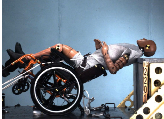
Figure 25. Peak rearward movement of ATD in manual wheelchair secured by traditional docking station
