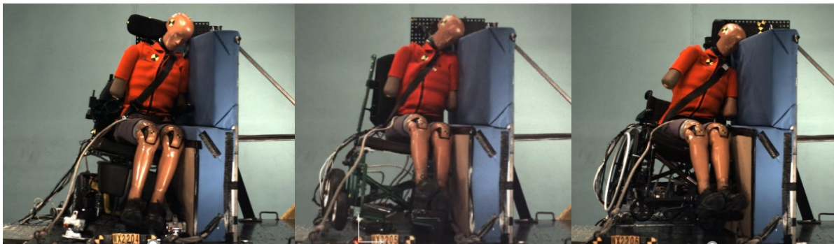
Figure 32. Comparison of peak lateral kinematics for power chair secured by 4-point strap tiedown (left), SWCB secured by traditional docking (center) and manual wheelchair secured by UDIG (right)
