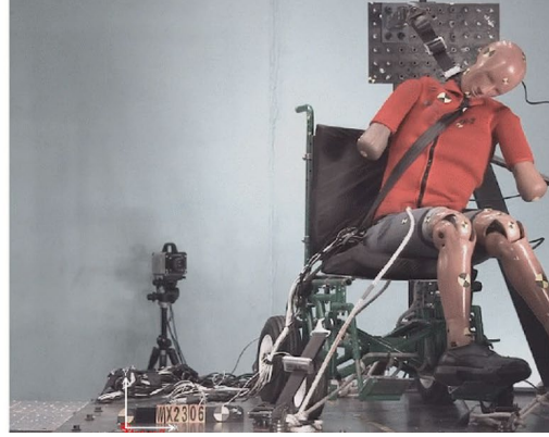
Figure 59. Peak excursion comparison of FE model of SWCSI secured by SWTORS to test WX2306 under nearside (center) impact
