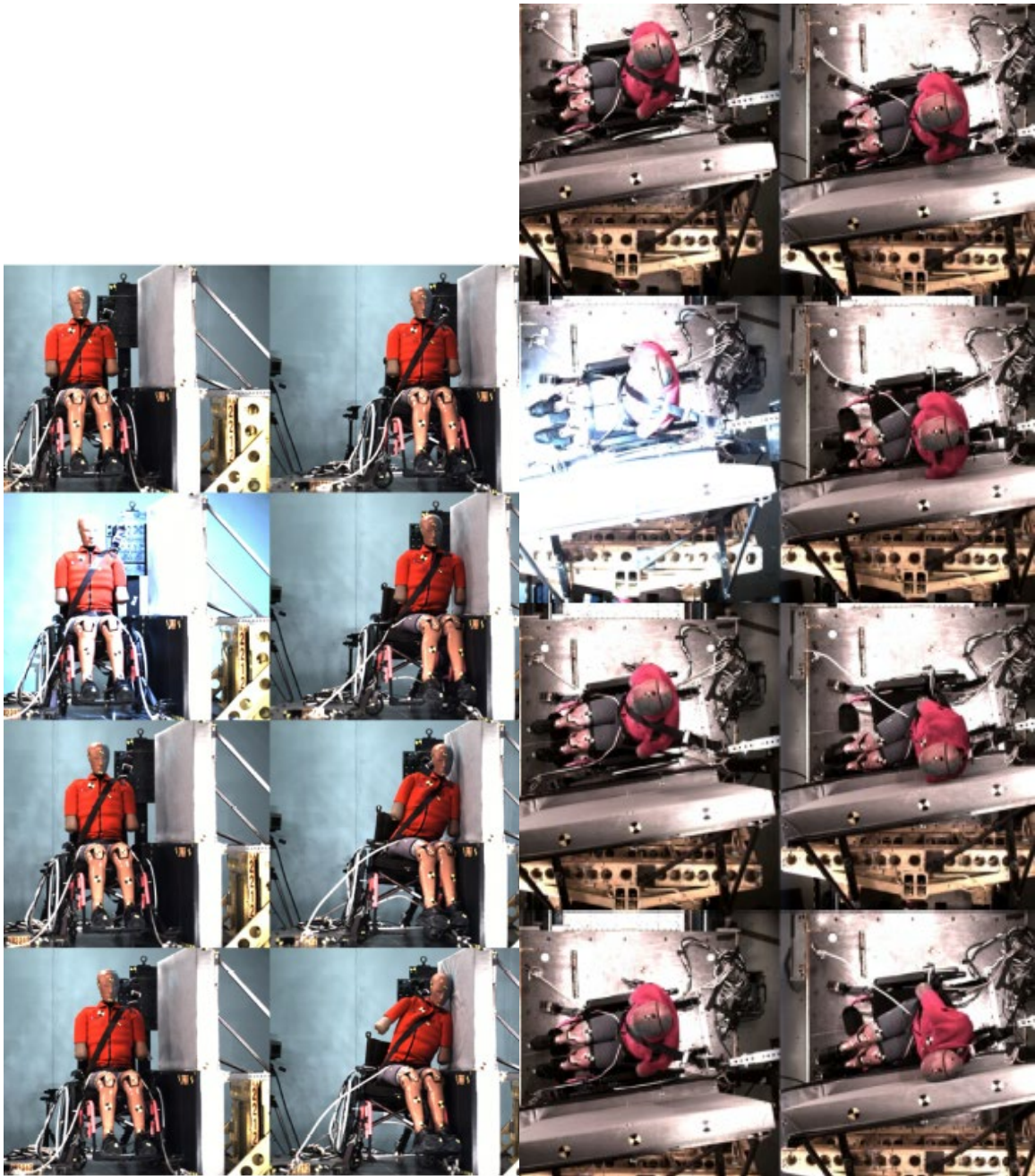
Figure F-1. Kinematics for WX2212, Ki Mobility+SWTORS, nearside with wall, from -20 to 120 ms every 20 ms
