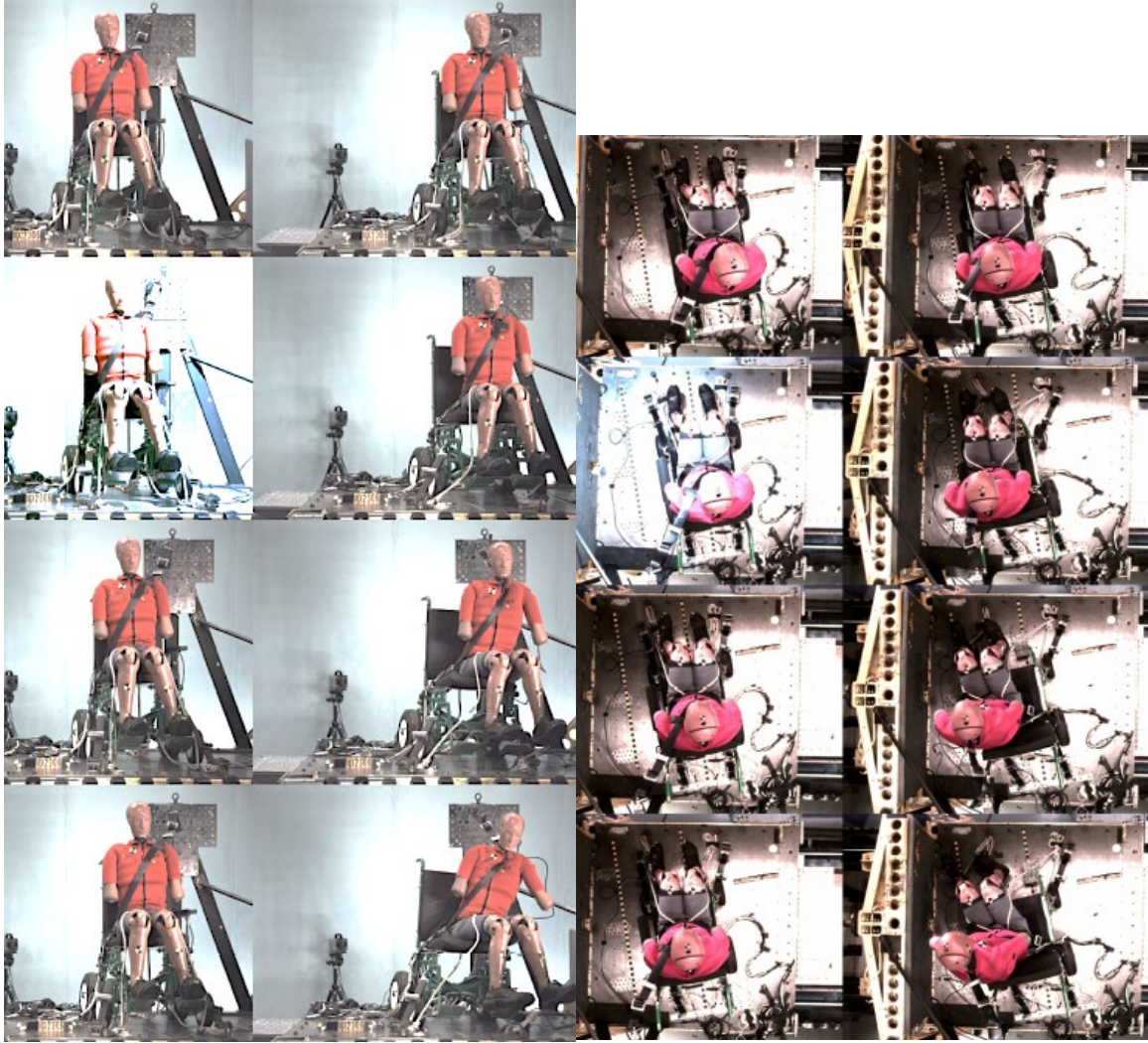
Figure F-12. Kinematics for WX2306, SWCSI+SWTORS, nearside (center) without wall, from -20 to 120 ms every 20 ms
