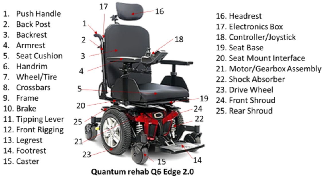
Figure C-1. Photo of power wheelchair and labeled components
