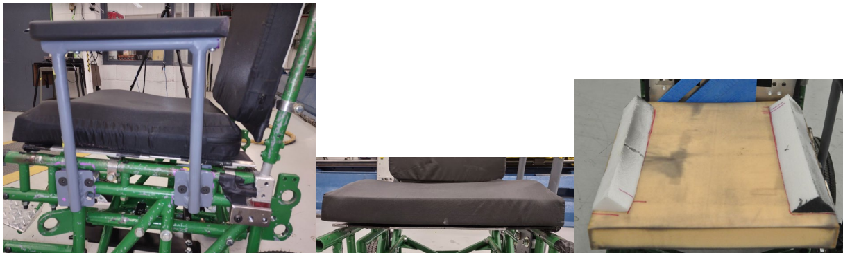
Figure 44. Modifications to turn SWCB into SWCSI: adding armrest, moving lap belt anchors forward, adding contour to flat seat
