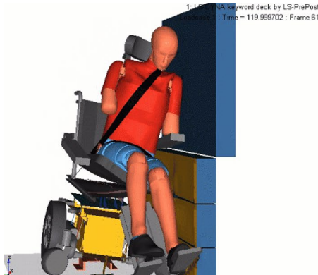
Figure 68. Peak excursion comparison of FE model of power wheelchair secured by traditional docking to test (WX2211) under nearside impact
