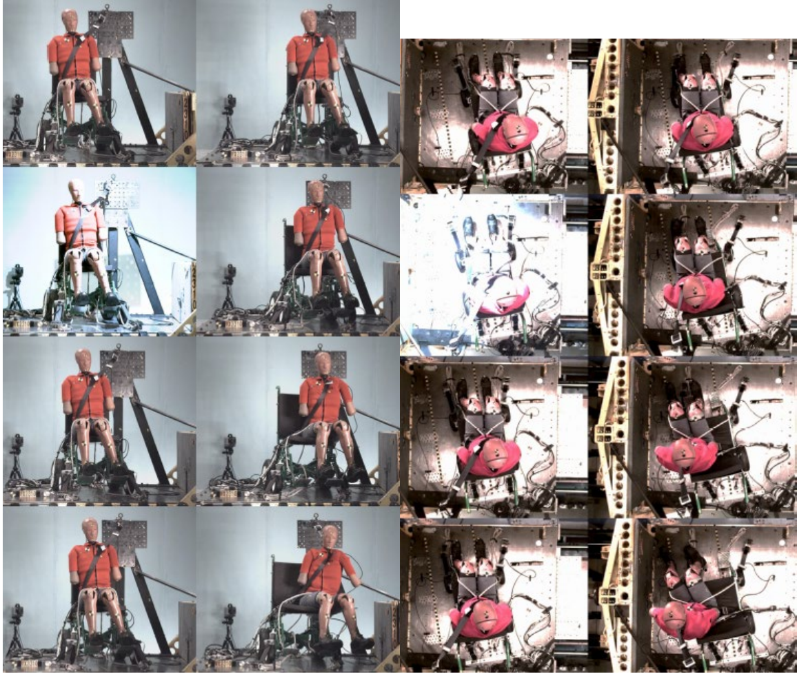
Figure F-10. Kinematics for WX2310, SWCB+SWTORS, nearside (center) without wall, from -20 to 120 ms every 20 ms
