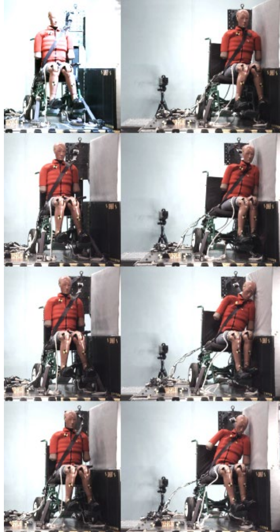
Figure F-6. Kinematics for WX2303, SWCSI+SWTORS, nearside with wall, from 0 to 140 ms every 20 ms
