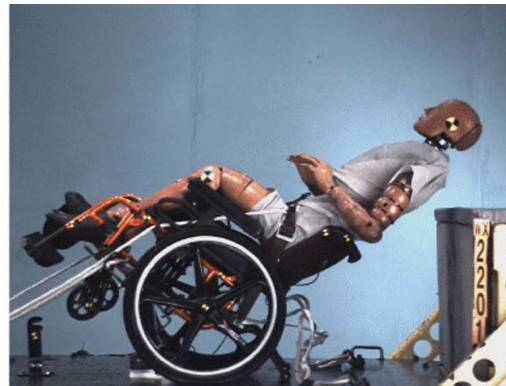
Figure 67. Peak excursion comparison of FE model of manual wheelchair secured by traditional docking to test (WX2201) under rear impact
