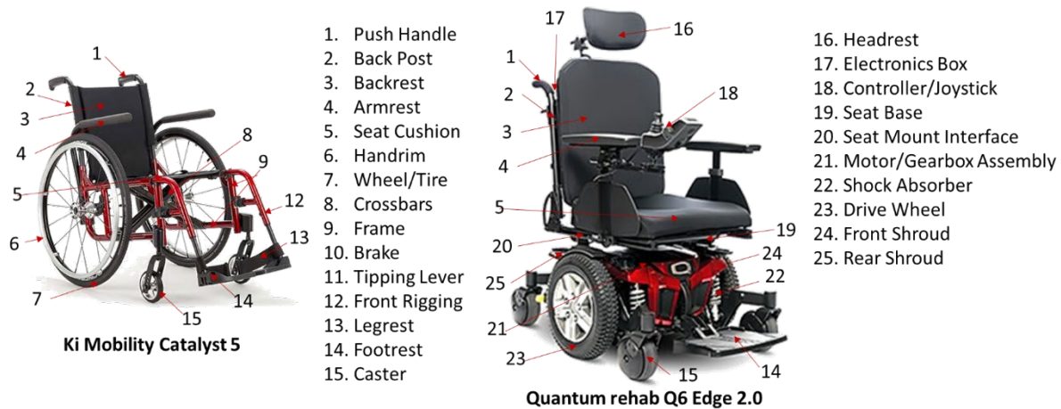
Figure 9. Components of a manual and a power wheelchair selected in this study
