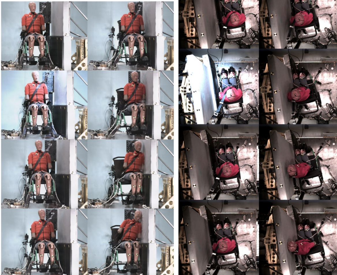
Figure F-3. Kinematics for WX2302, Leggero+SWTORS, nearside with wall, from -20 to 120 ms every 20 ms
