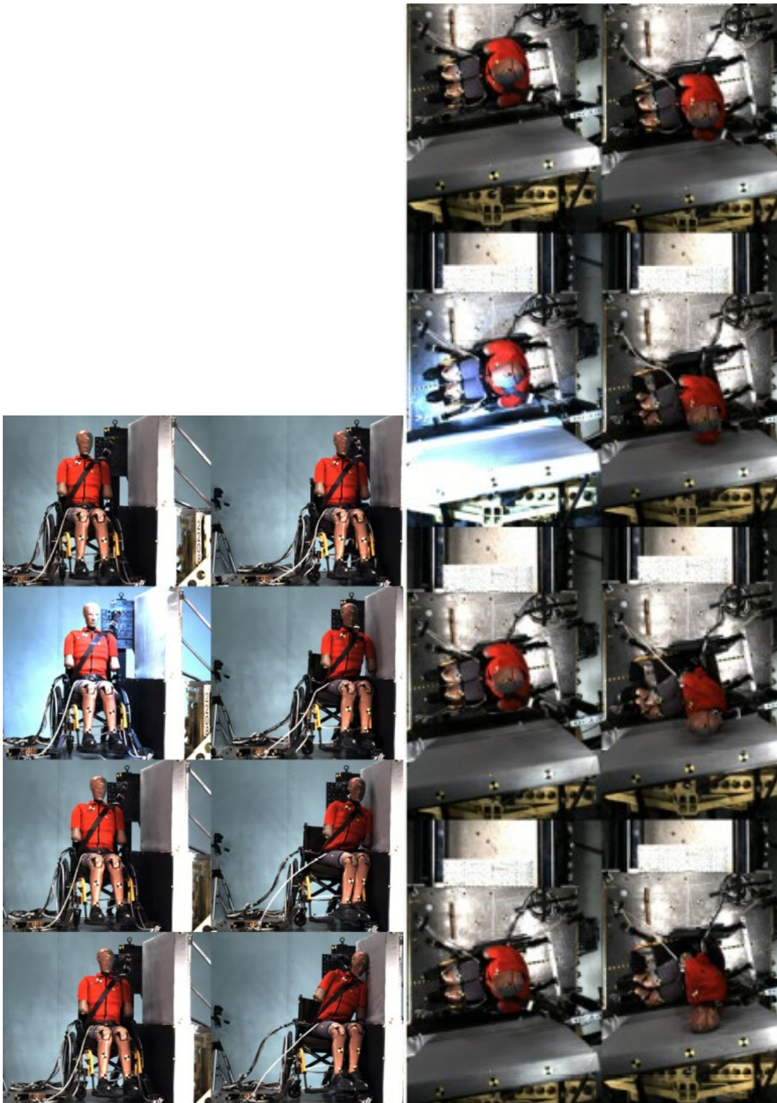
Figure F-2. Kinematics for WX2208, Quickie 2+SWTORS, nearside with wall, from -20 to 120 ms every 20 ms
