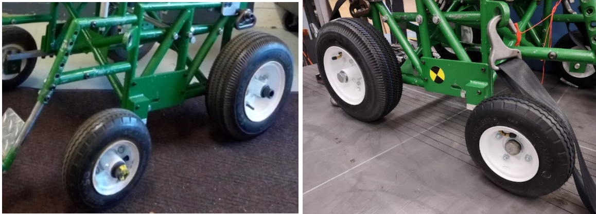
Figure 42. Original (left) and revised (right) wheels and bolts used on SWCB
