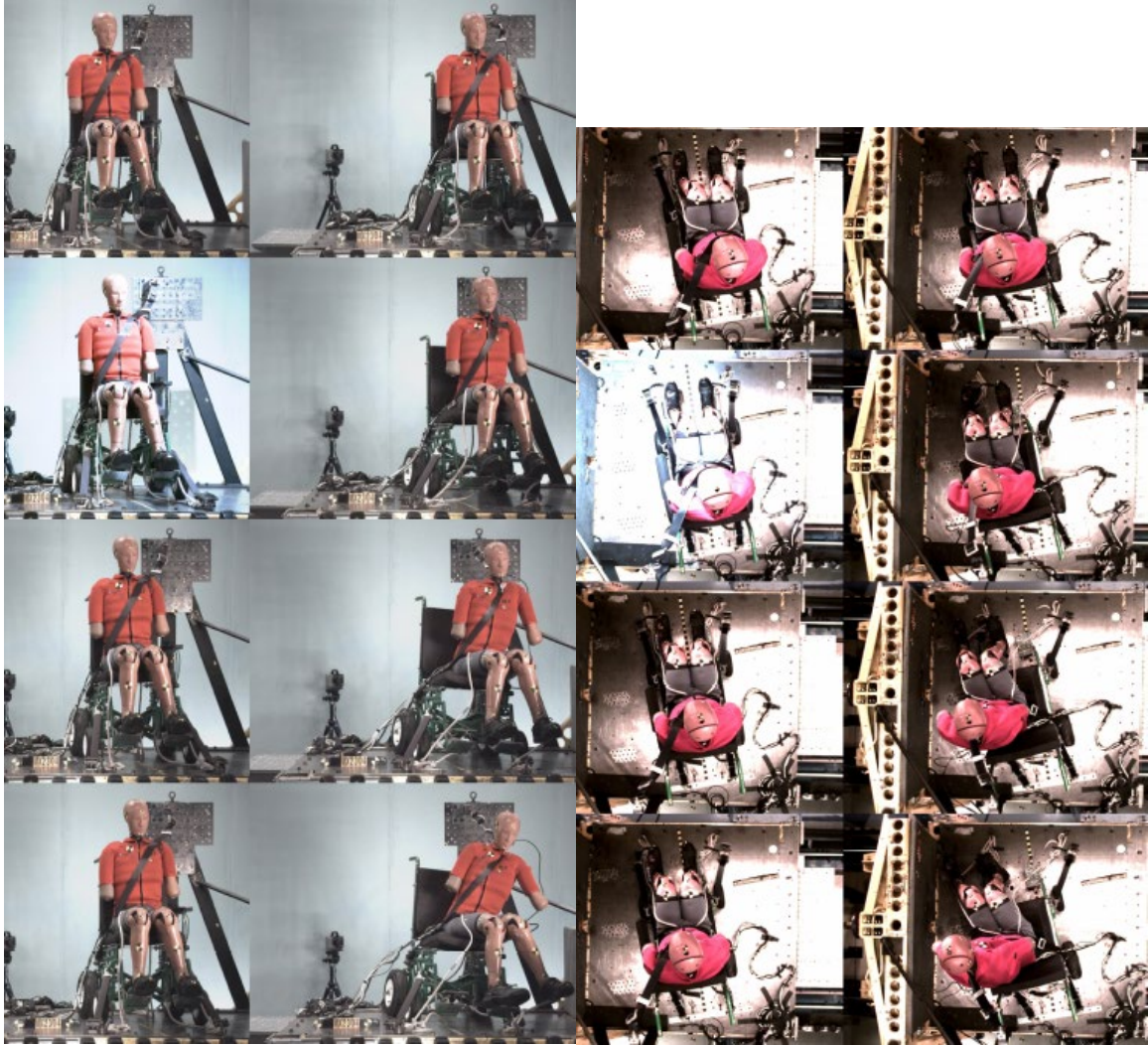
Figure F-11. Kinematics for WX2304, SWCSI+SWTORS, nearside (center) without wall, from -20 to 120 ms every 20 ms
