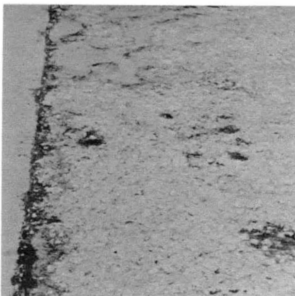
Figure 5-2 Light scale. Scale depth is less than \frac{1}{4} ".
