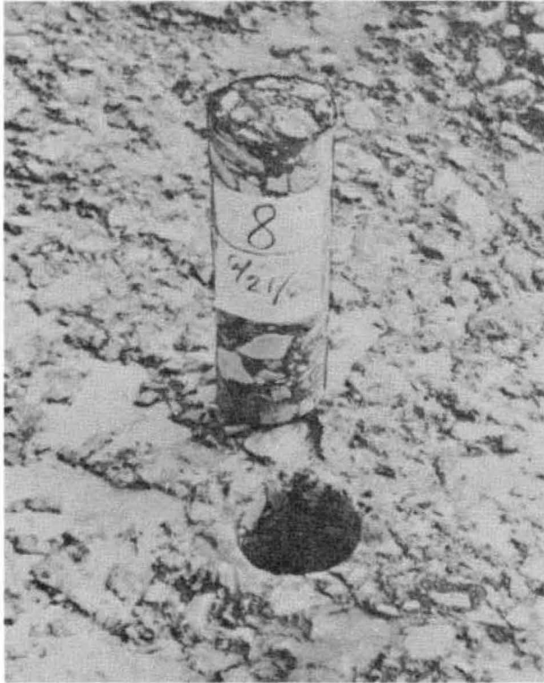
Figure 5-4. Heavy scale. Note depth is between \frac{1}{2} " and 1". Note virtually complete exposure of coarse aggregate.
