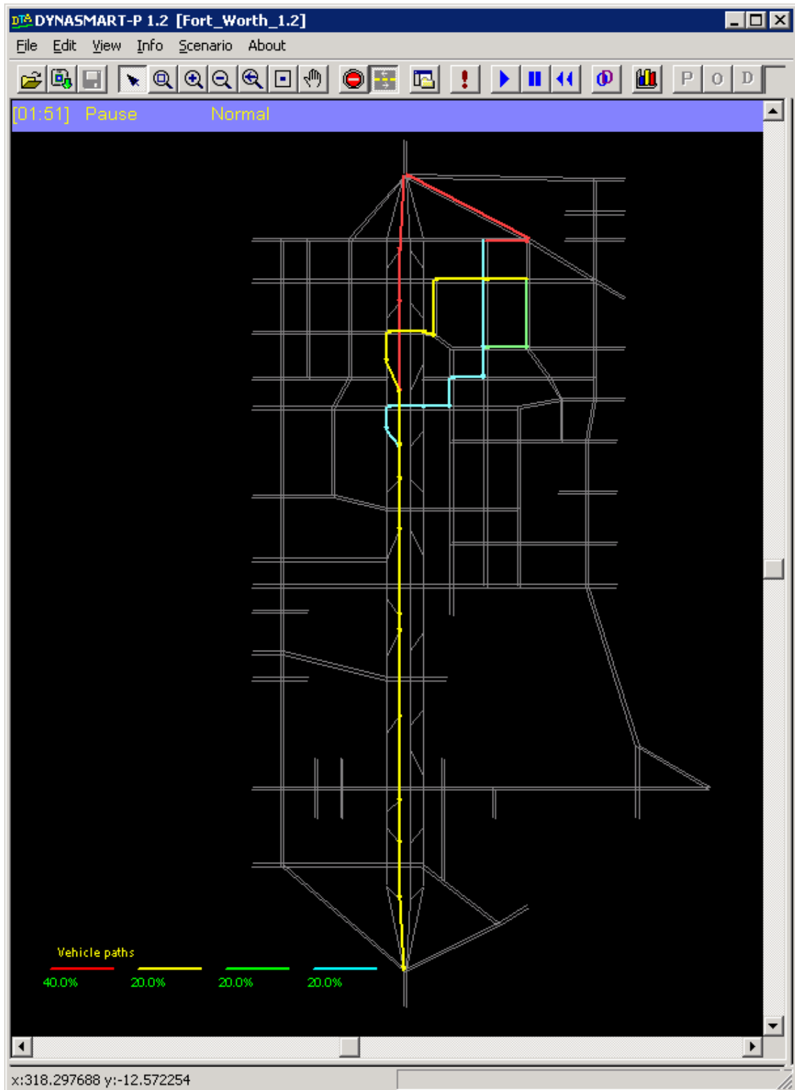
Figure 6-90. Vehicle paths as displayed on the GUI after clicking the yellow path legend
