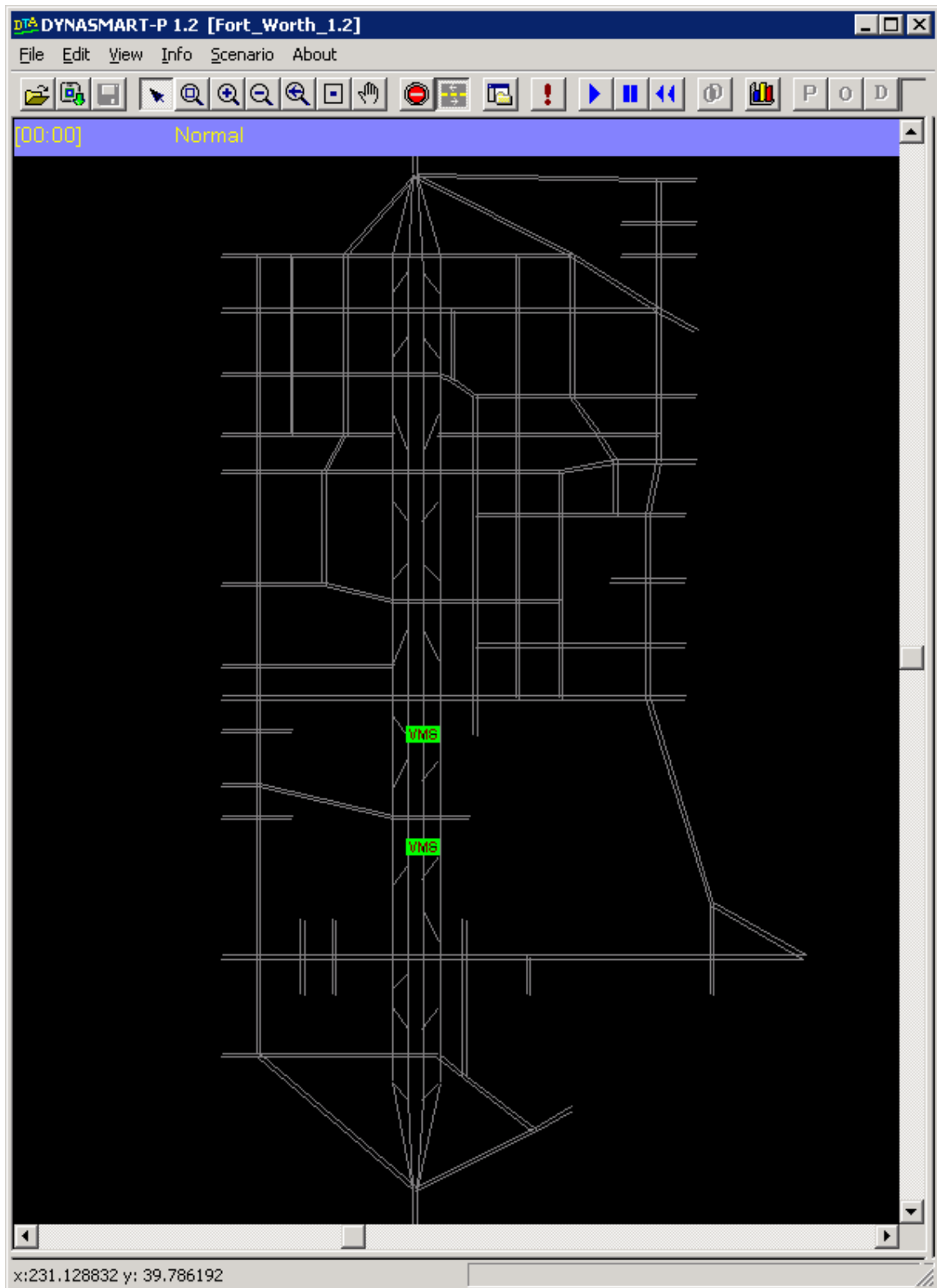
Figure 6-42. VMS signs as shown on GUI
