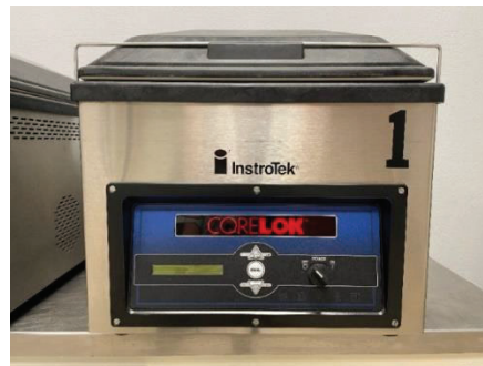
Figure 16. A CORELOK Machine Used in Specific Gravity Measurements.
