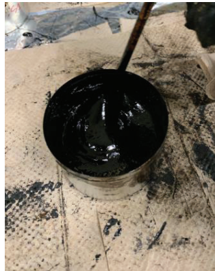
Figure 15. RAP Blending With Virgin Plant Binders.
