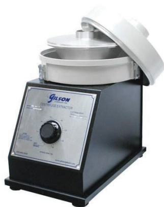
Figure 13. Centrifuge Extractor for Asphalt Binder Extraction Process.
