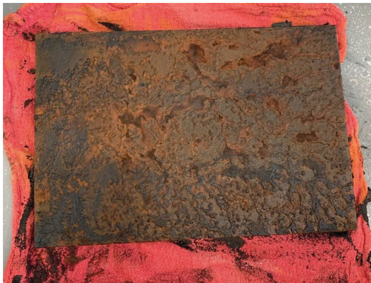
Figure 70. Horizontal Weathering Steel Plate After Eight Weeks
