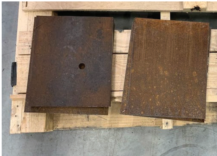
Figure 67. Bare Weathering Steel Plates
