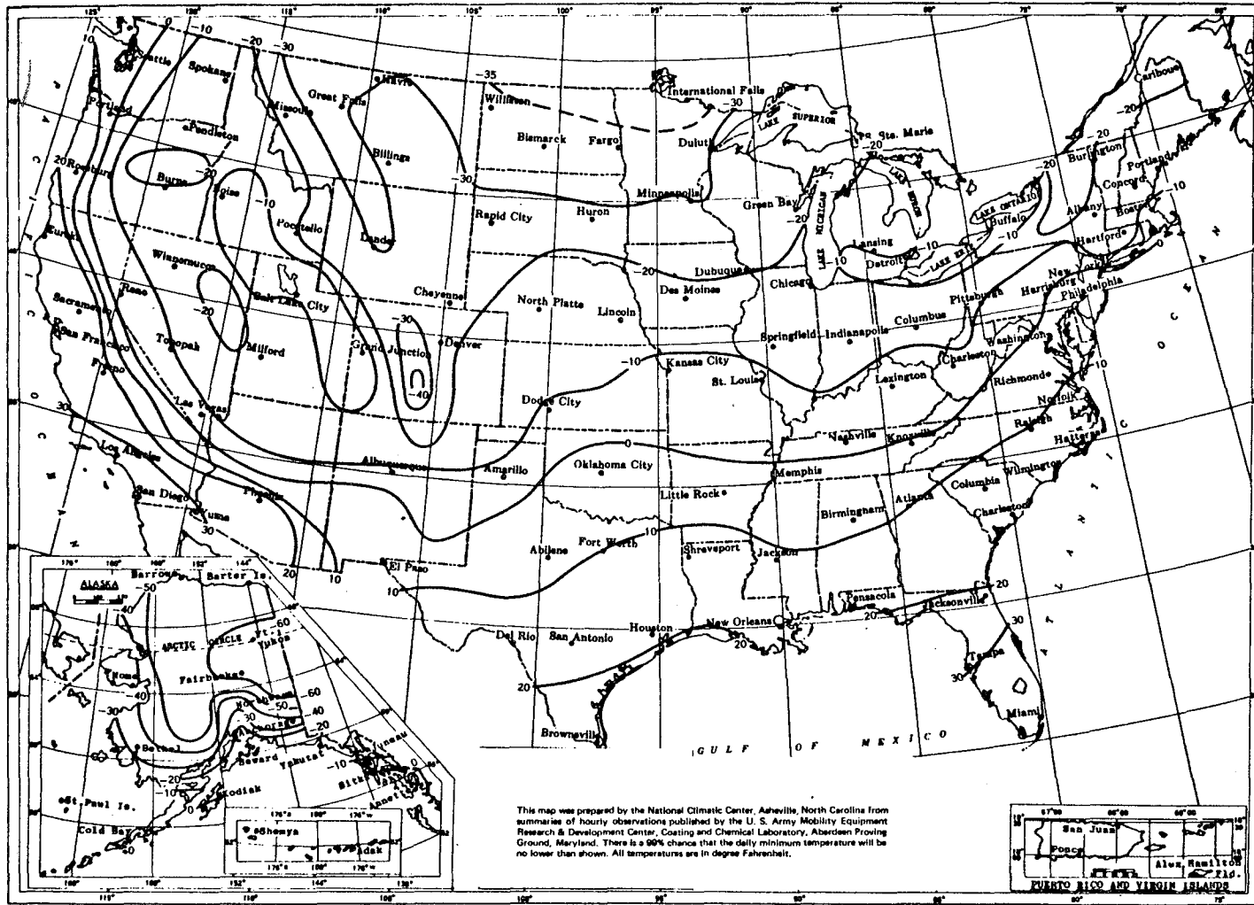
FIGURE 1.5.4.1 - ISOLINES FOR FIRST-PERCENTILE MINIMUM TEMPERATURES, the basis for determining the lowest anticipated service temperature (LAST) for fracture critical members (FCMs).
