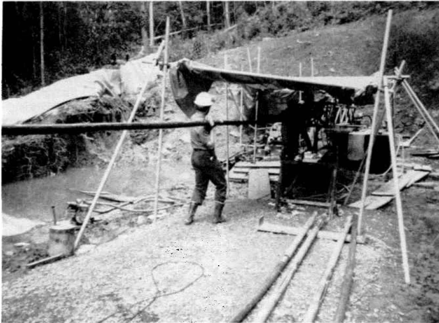
Starting the subsurface exploration sensor probes into the 305 m (1,000 ft) long horizontal borehole.
