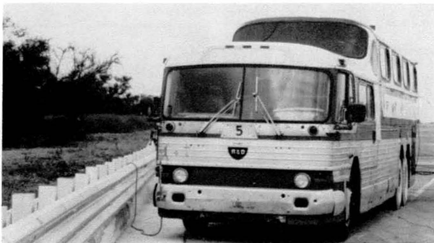
Self-restoring bridge rail for retrofit applications.
