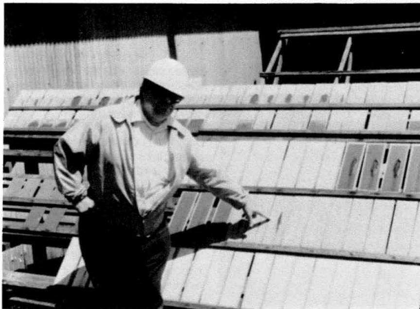
Rating some of the 5,000 panels on outdoor exposure as part of the PACE project.
