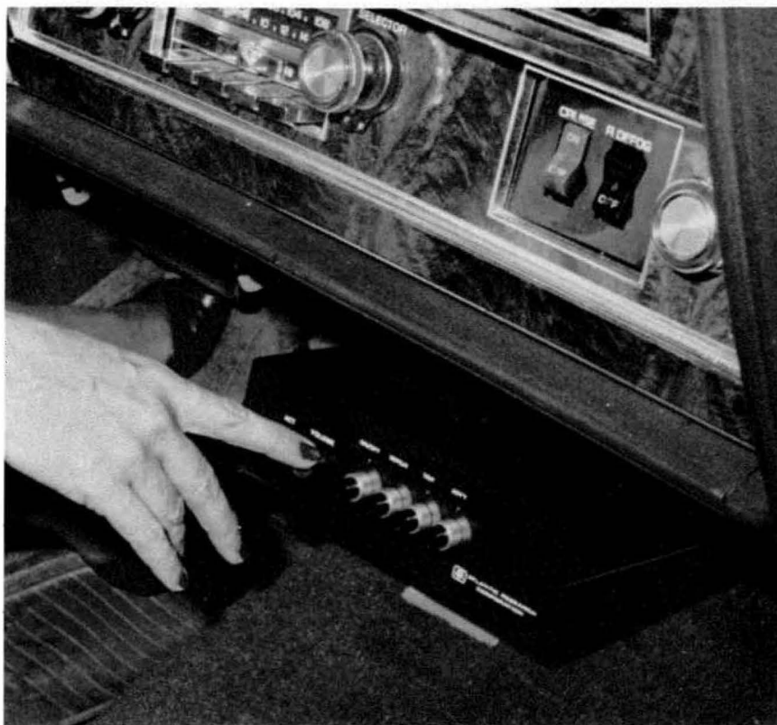
In-vehicle receiver for an Automatic Highway Advisory Radio system.
