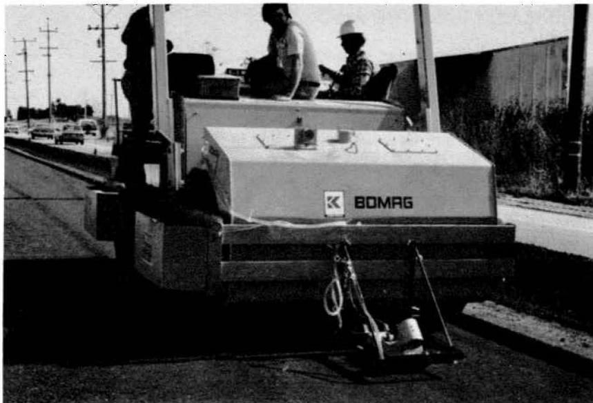
Roller-mounted nuclear gage for monitoring asphalt concrete density and temperature.
