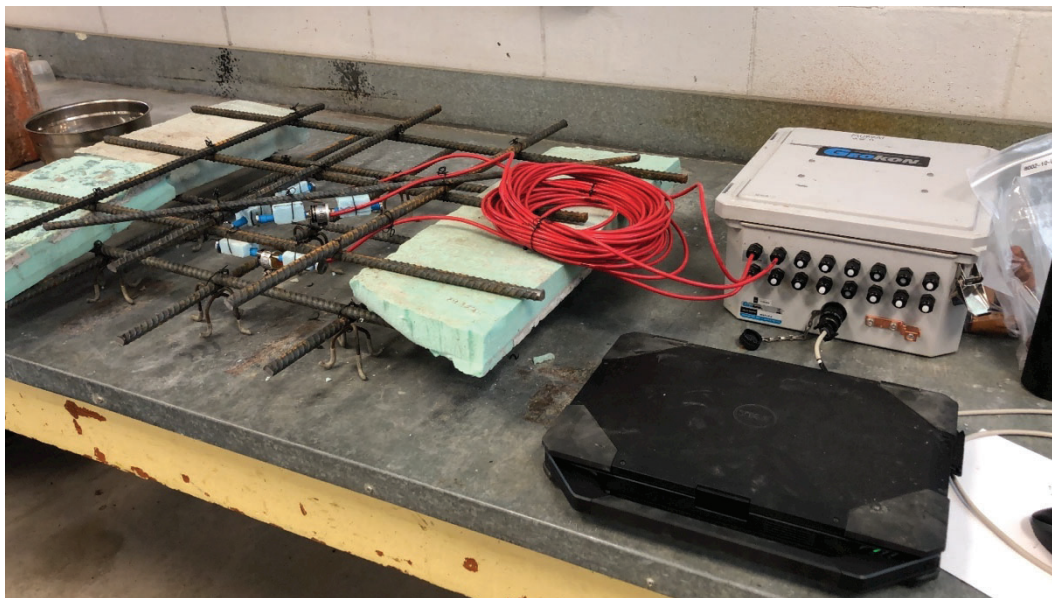
Figure 10. Data Acquisition Set-Up Showing Mock-Up VWSG Rosette and Computer
