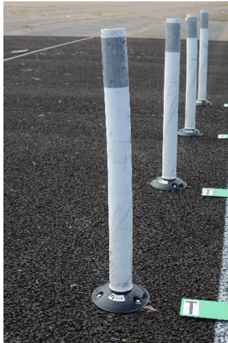
Figure 3.61. 607531-02-10 Sample (Powers Wedge-Bolt).
