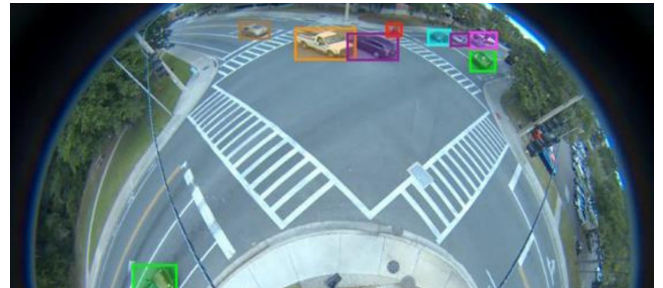
Fisheye camera image of an intersection with bounding boxes on detected objects.
