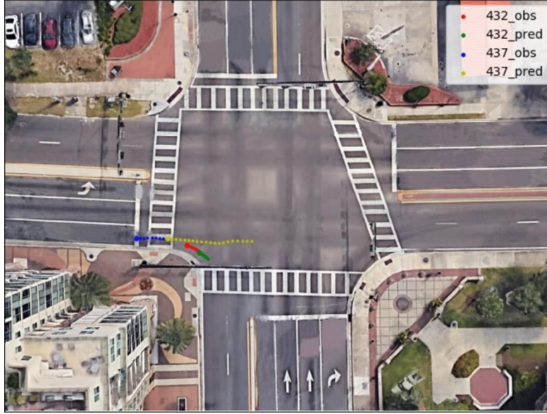
Figure 8-9. Visualizations of the output from trajectory prediction algorithm. As shown in the bottom left corner, the red and blue trajectories represent the observed trajectory of Cars 432 and 437 respectively; the yellow and green ones represent the predicted trajectories.
