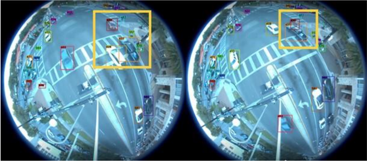
Figure 8-7. Two snapshots of the surveillance video at W University Ave & NW 13 th St showing a collision. A collision happens between vehicle 432 and vehicle 437. The left one is before collision, and the right one is when the collision occurs.
