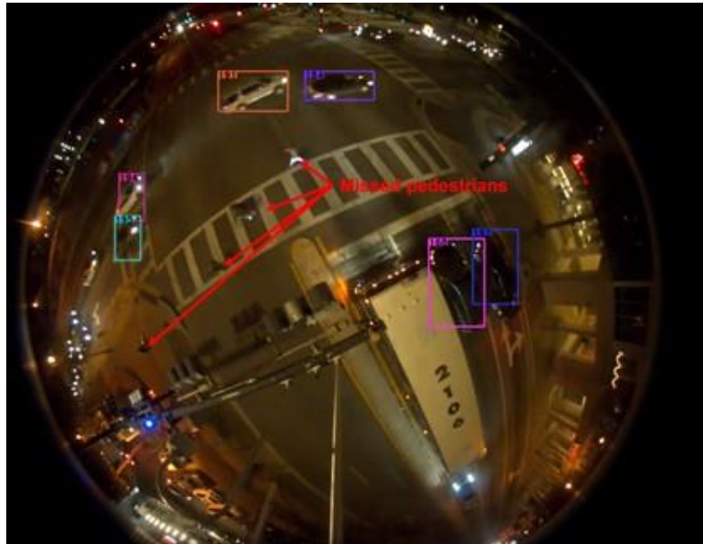
Figure 4-8. Examples of nighttime fisheye frames where the detector fails to detect pedestrians on the crosswalk.
