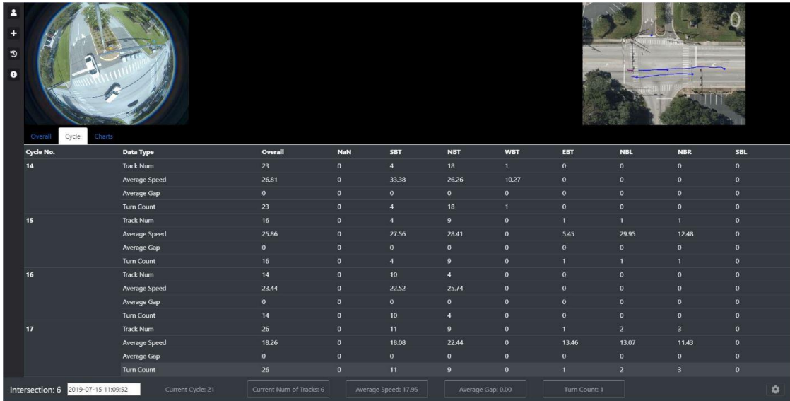
Figure 5-8 The cycle tab of the detailed statistical data shows the statistics data aggregated by signal cycles and displayed by cycle counts.
