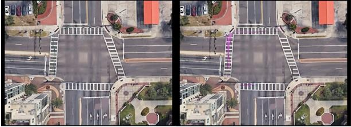
Figure 4-9. Comparisons between nighttime pedestrian detection using fisheye cameras (left) and LIDAR sensors (right) at the same time period. It is observed that pedestrian trajectories of the fisheye cameras are generally discontinuous, i.e., the whole trajectory of a single pedestrian might be broken down to several small trajectory segments due to the difficulty of consistently tracking and detecting a pedestrian at night. Trajectories from LIDAR videos are more complete. And it is able to detect pedestrians that are missed/dropped in the fisheye cameras.
