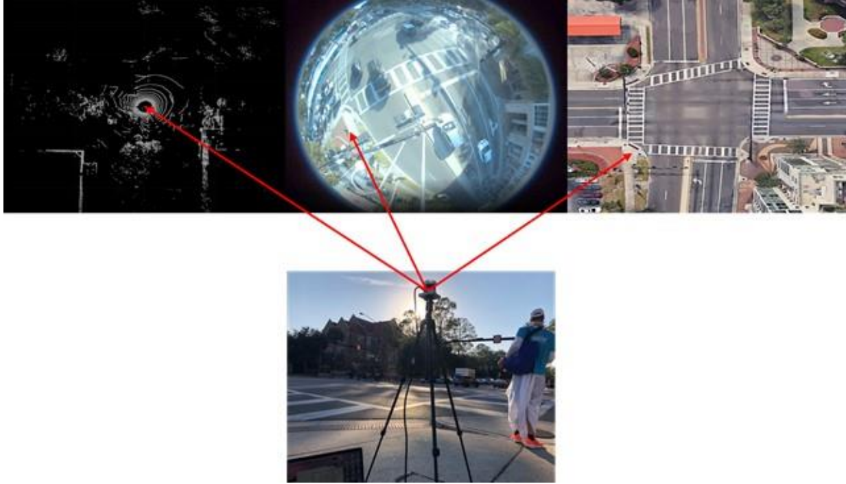
Figure 3-4. Another LIDAR setup. The LIDAR sensor is installed at the busy intersection of W University Ave at 13 th St in Gainesville, FL, to collect bicyclist data.
