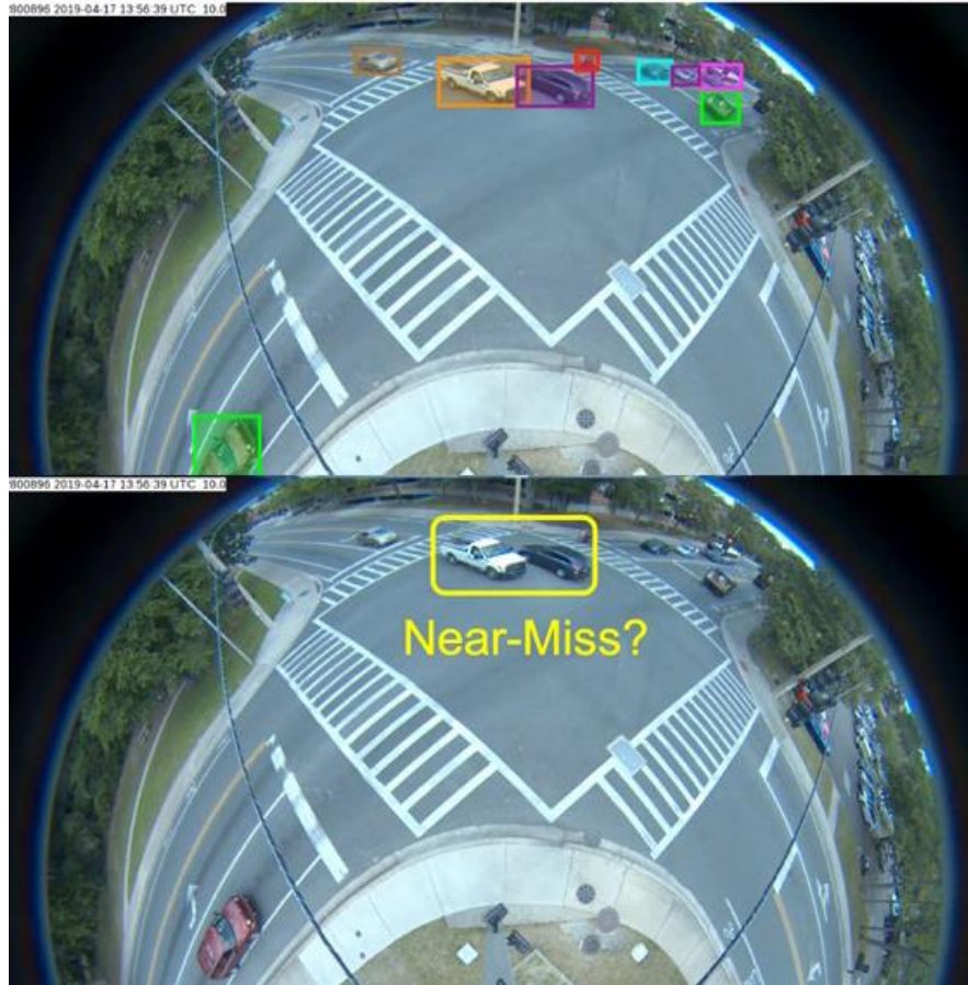
Figure 1-1. Top: Fisheye camera image of an intersection with bounding boxes on detected objects. Bottom: Bounding boxes indicate a near-miss, but this is a false identification. The two vehicles are driving through the intersection in opposite direction.
