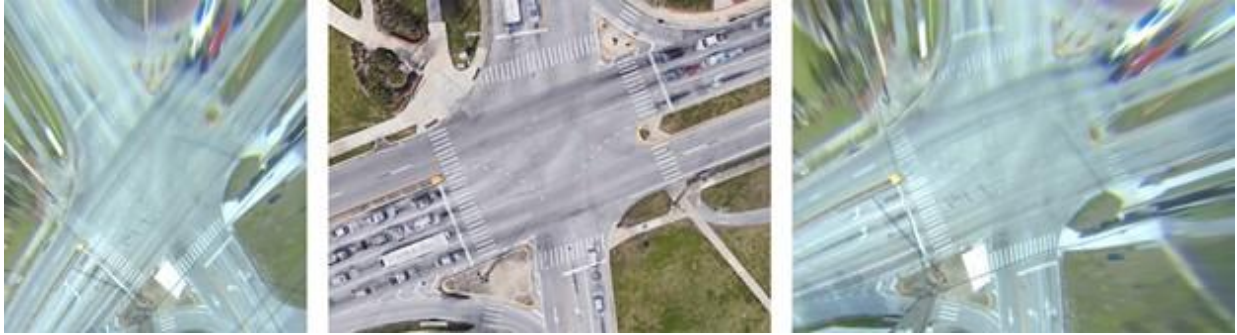
Figure 1-11. Left: Image after distortion correction. Middle: Google-Map reference. Right: Image after TPS transform
