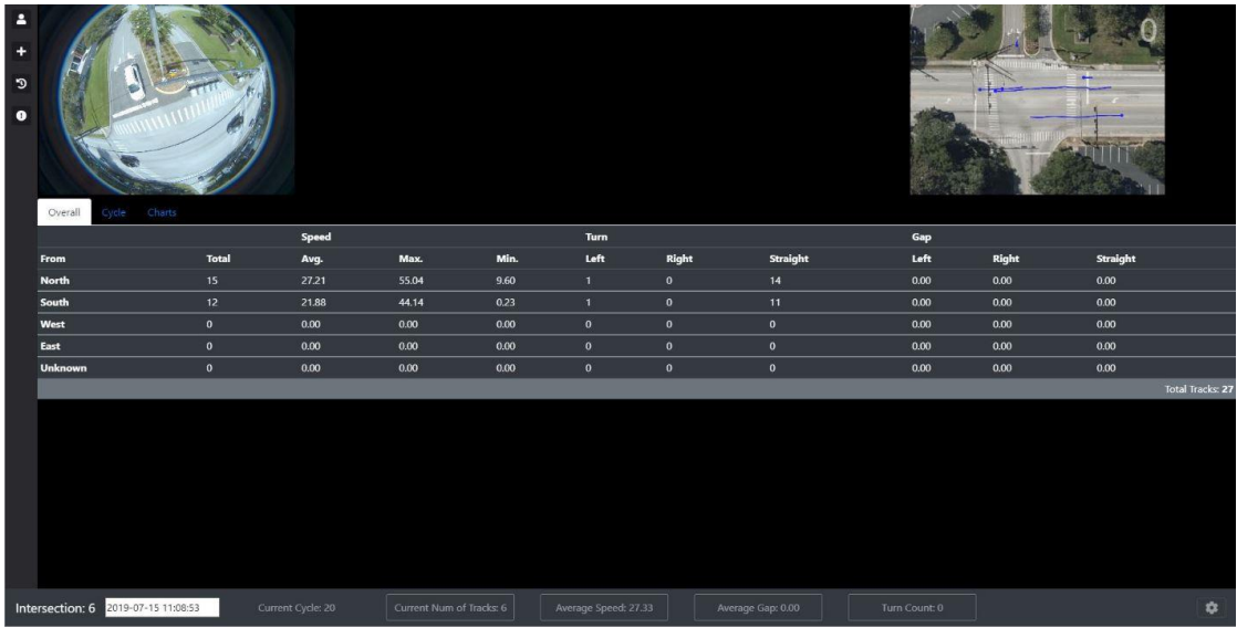
Figure 5-7. Clicking on the statistics table on the main page toggles the display to more statistical details. These are organized into three tabs, namely, Overall, Cycle, and Charts. We see the overall statistics here, for speed, gap and turn movement counts.
