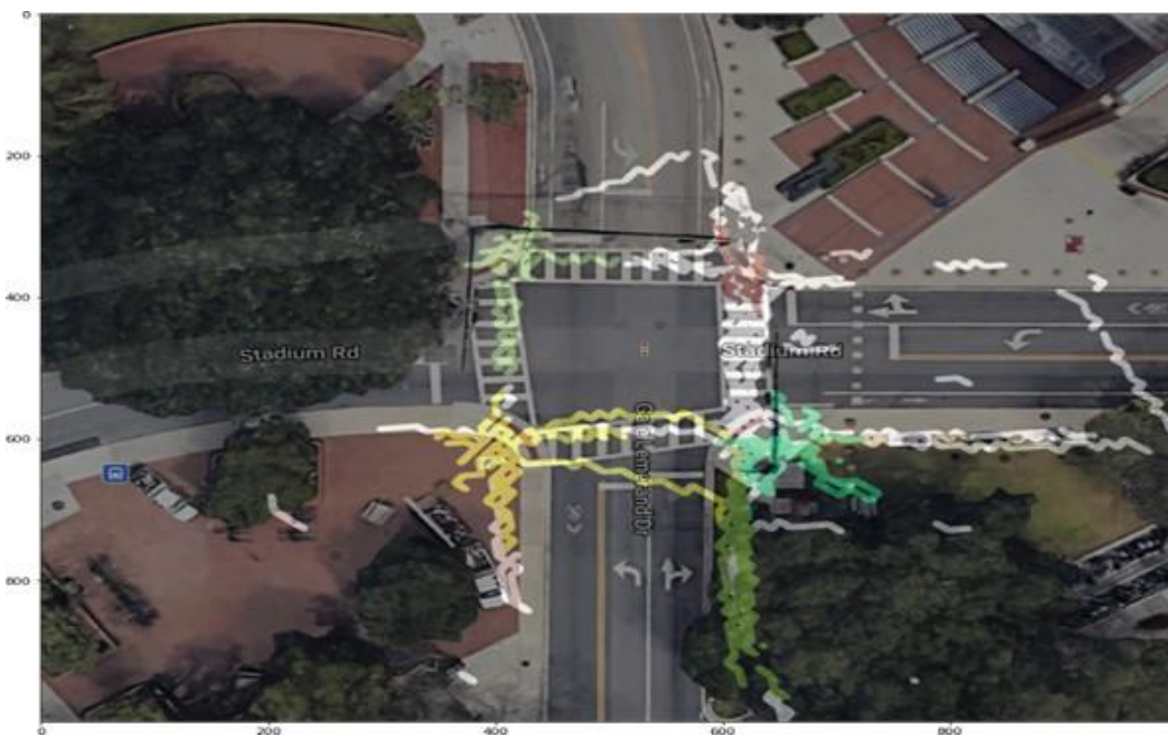
Figure 3-13. Trajectory clustering for pedestrians, generated by HDBSCAN Clustering
