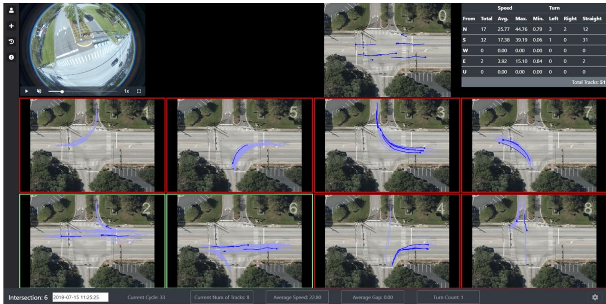
Figure 5-5. Interface for showing the tracks. The video from the fisheye camera is at the top left corner. This is followed by an unwarped image of the intersection and the trajectories as represented by a moving dot. The statistics of the trajectories on the intersection are captured in the table on the top right side. The trajectories are partitioned into phases and displayed in the eight windows. The setting options and average statistics about the trajectories are present at the bottom.
