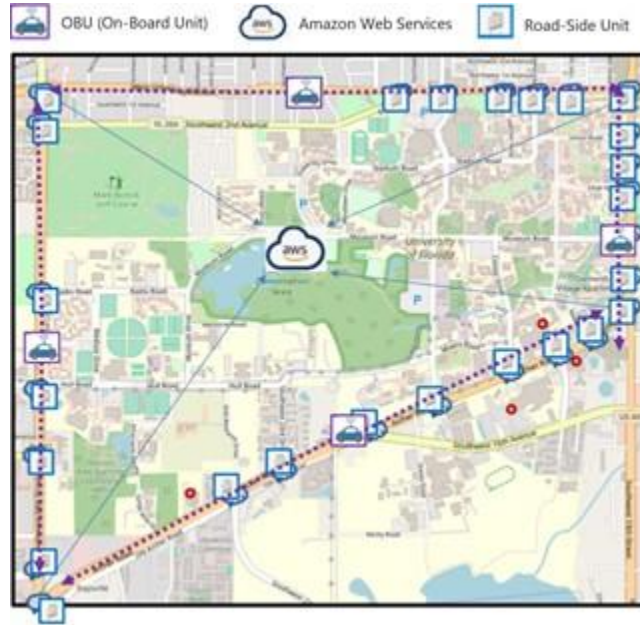
Figure 3-1. Trapezium+ = Trapezium after SPaT project (data sharing and ATSPM; upgraded Linux-based 'ATC' controllers; ATSPM data sharing to University of Florida and third party (TTS, TrafOps, Live Traffic Data, Connected Signals); Siemens DSRC radios with MAP and SPaT broadcast; emergency vehicle pre-emption and vehicle OBUs). The solid arrow lines denote that all collected data will be sent to AWS cloud for data storage.
