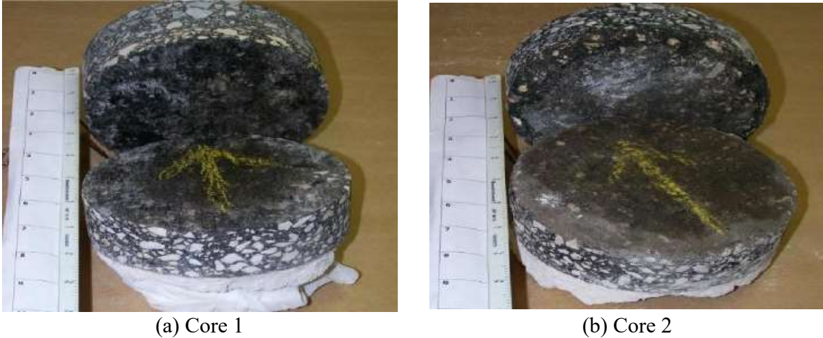
(a) Core 1 (b) Core 2 Figure 1-4 Cores taken from areas near Slippage Location 2 (Photos courtesy of FDOT district engineers).
