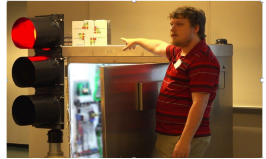
A member of the University of South Florida's Center for Urban Transportation Research showcases a cyberattack on a connected vehicle roadside unit (potentially a traffic signal system) via an onboard unit.
