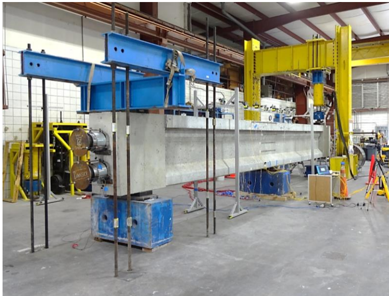
Figure E.23 Beam specimen NB-2 inside test frame and tie-down
