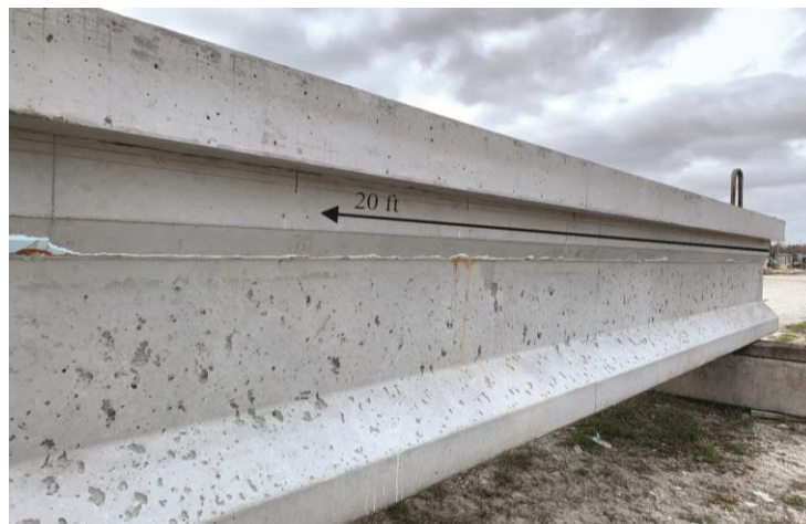
Figure 5.18 Formation of crack on specimen SS-2 at a distance of 20 ft from west end (north side)
