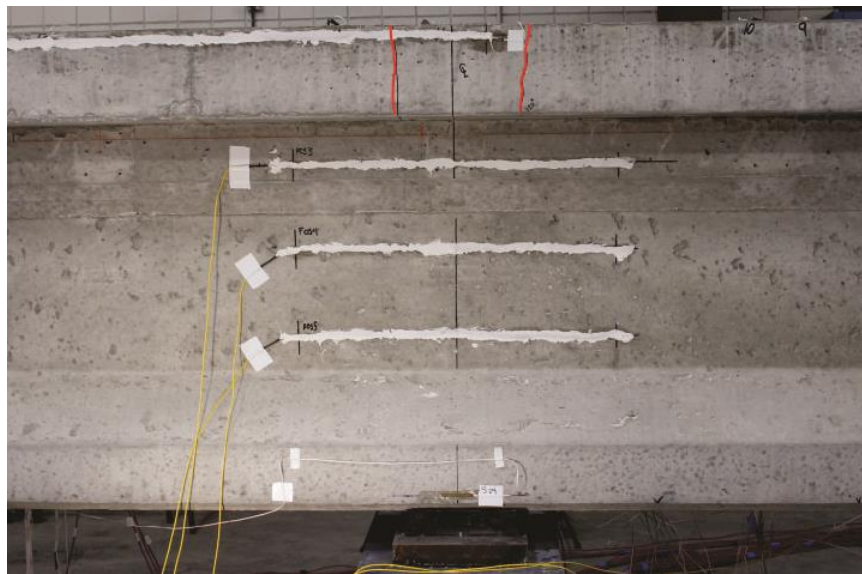
Figure 8.63 Specimen NB-1: First observed cracks (marked in red) at P = 120 kip
