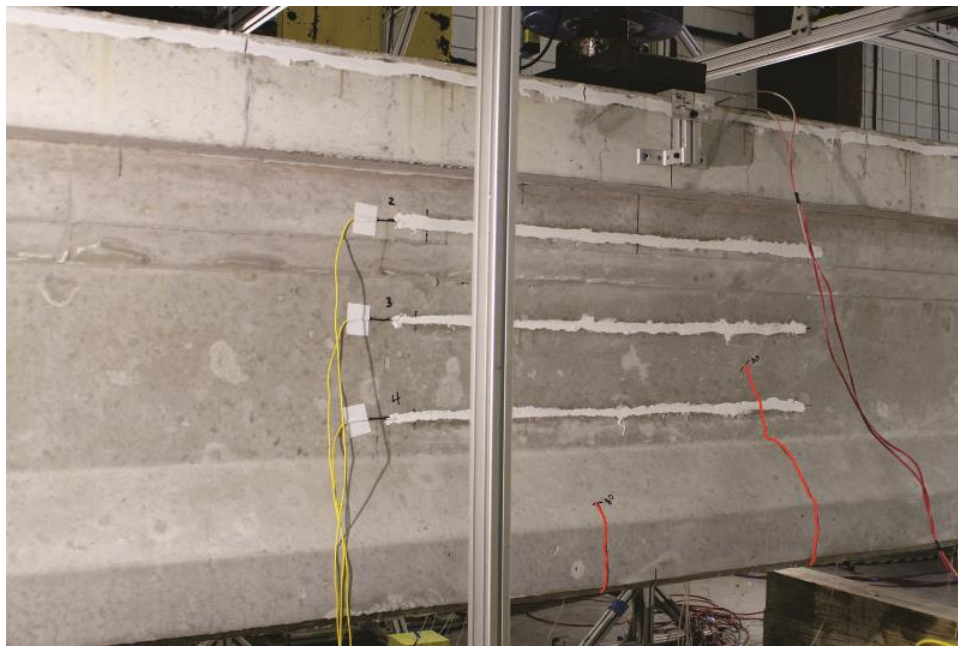
Figure C.39 Specimen SS-4: first observed cracks (marked in red) at P = 80 kip on east side
