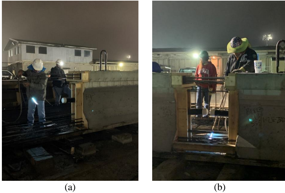
Figure 5.17 Detensioning of SS specimens at (a) east end of prestressing bed and (b) between specimens SS-2 and SS-3
