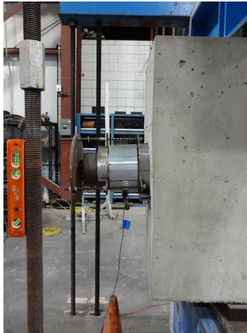
Figure 7.18 Geokon hollow-core load cell installed at dead end of beam specimen NB-1
