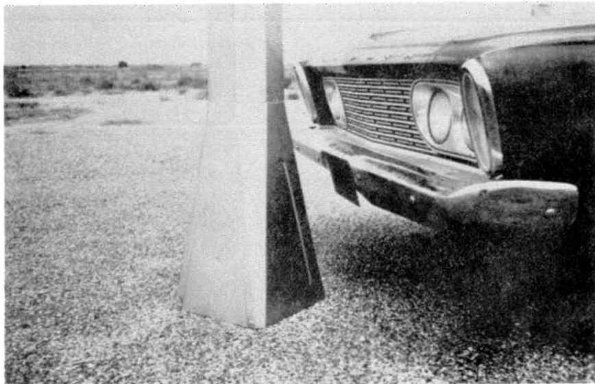
Figure 16. Stainless steel base and support.
