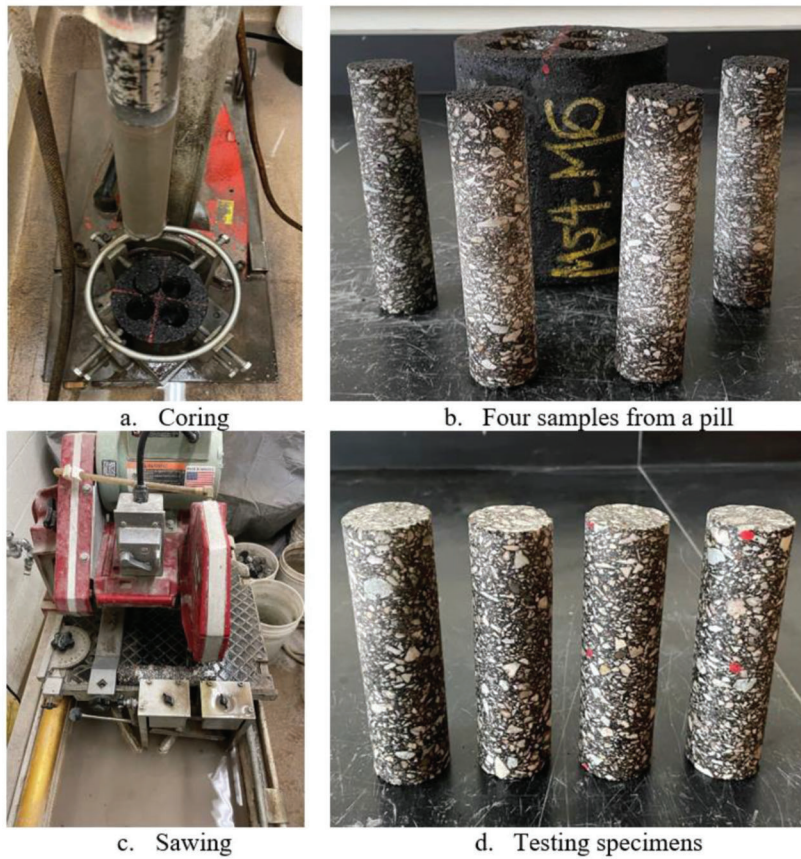
Figure 3.2 Testing specimen fabrication process.
