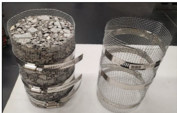
Figure 3.1 Wire mesh holder preventing the collapse of the samples during aging.
