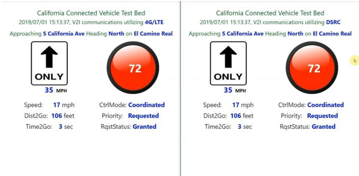
Figure 18 Side-to-Side HMI Dashboard with DSRC and 4G LTE
