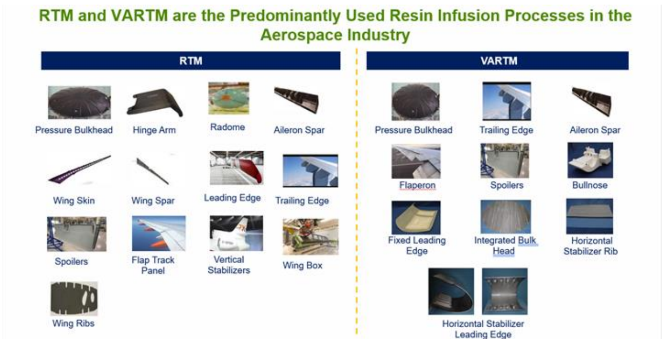
Figure 38. Aircraft parts comparison for RTM and VARTM processes (from Lucintel)
