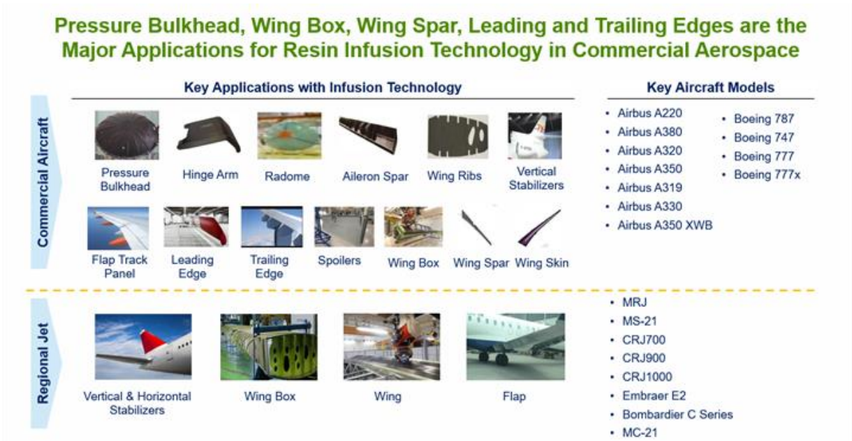
Figure 37. Aircraft parts best suited for resin infusion processes (from Lucintel)
