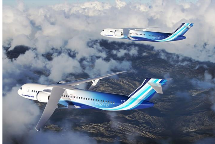
Figure 30. Concept of Boeing Transonic Truss-Braced Wing (TTBW) configuration Reproduced with permission from Composites World and Boeing
