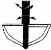
Mixing tool for constructing Lime Cement Columns™.
