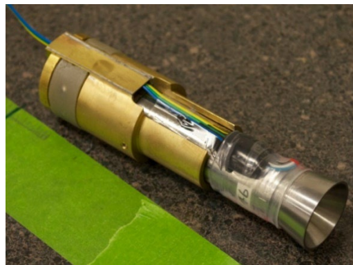
Figure 3.13: (a) Schematics and Detailed Components of an MDD Assembly; and (b) Photograph Showing an LVDT Module
