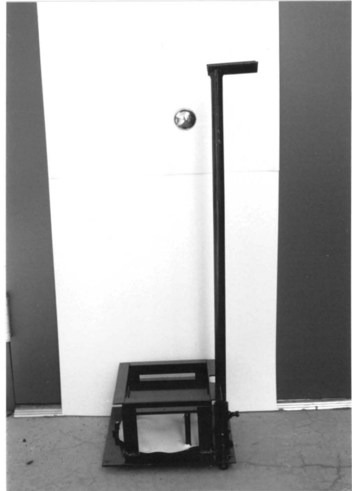
Figure 11. Modified Vialit test used by University of Nevada-Reno. (39)
