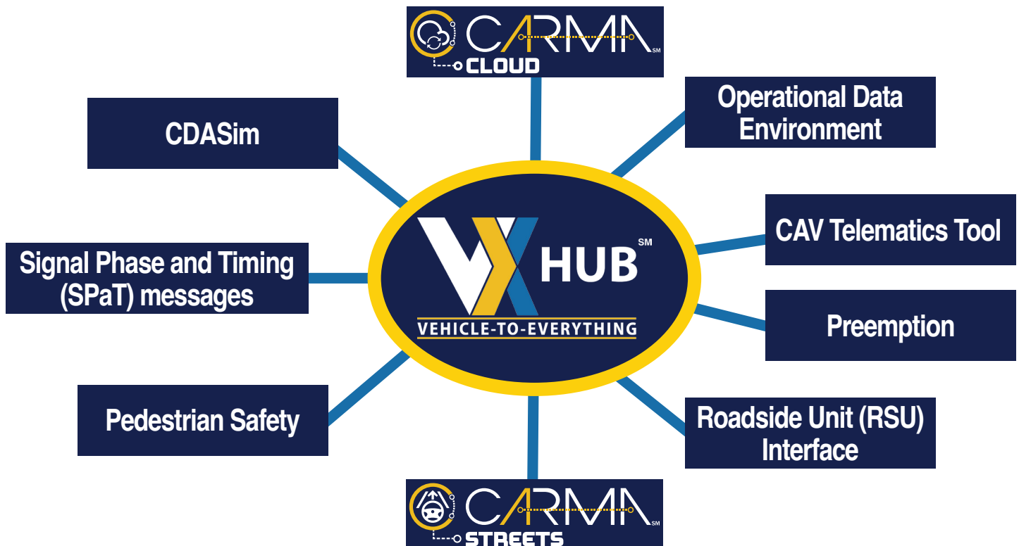
Figure 1. Image. Functionalities of V2X Hub.
