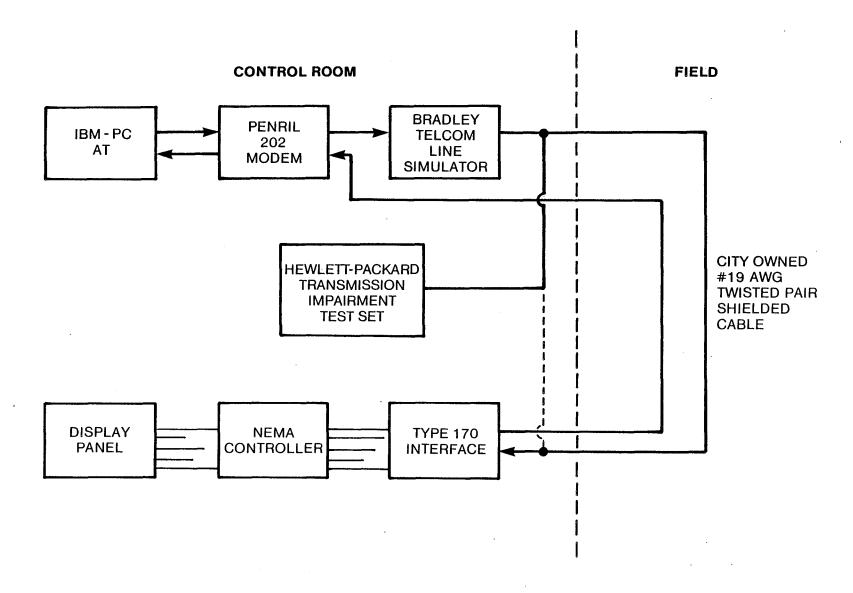
Figure 4. Test Configuration Block Diagram.
