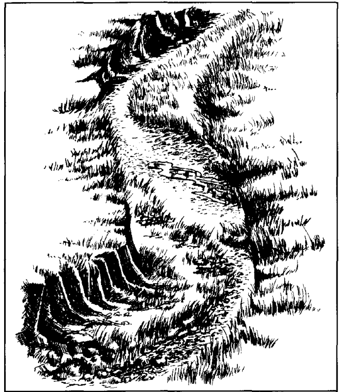
Figure 33b. Channel treatment reduces runoff velocities and initiates deposition of sediment fans which evolve into point bars as wetland vegetation stabilizes the accumulating sediments.
