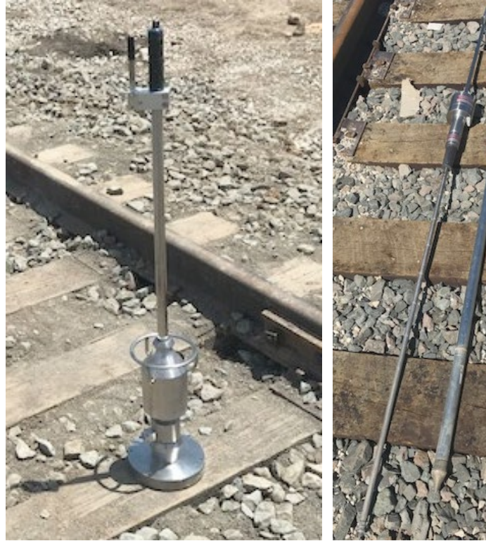
Figure 6. Lightweight deflectometer (left) and dynamic cone penetrometer (right).
