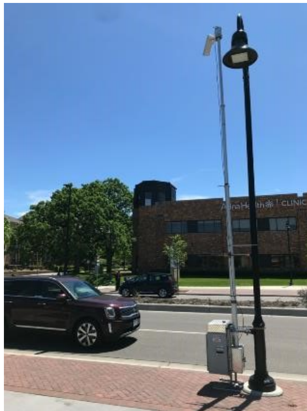
Figure B.1: TIM unit deployed showing water tight enclosure at bottom containing microcomputer and batteries as well as extendable mast and camera.
