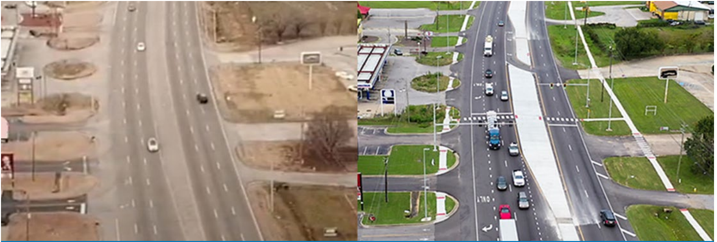
Aerial photos of Alabama's West South Boulevard before (left) and after (right) pedestrian safety improvements such as reduced lanes, a raised median, and lighting installation were made. Watch a video about the project to learn more.
